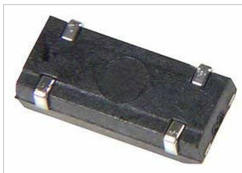
Figure 1: ABRACON ABS25-32.768KHZ-6-T Low Frequency Crystal. This image shows a small, black, rectangular surface-mount electronic component with four metallic contacts on its sides, designed for precise timing applications.
