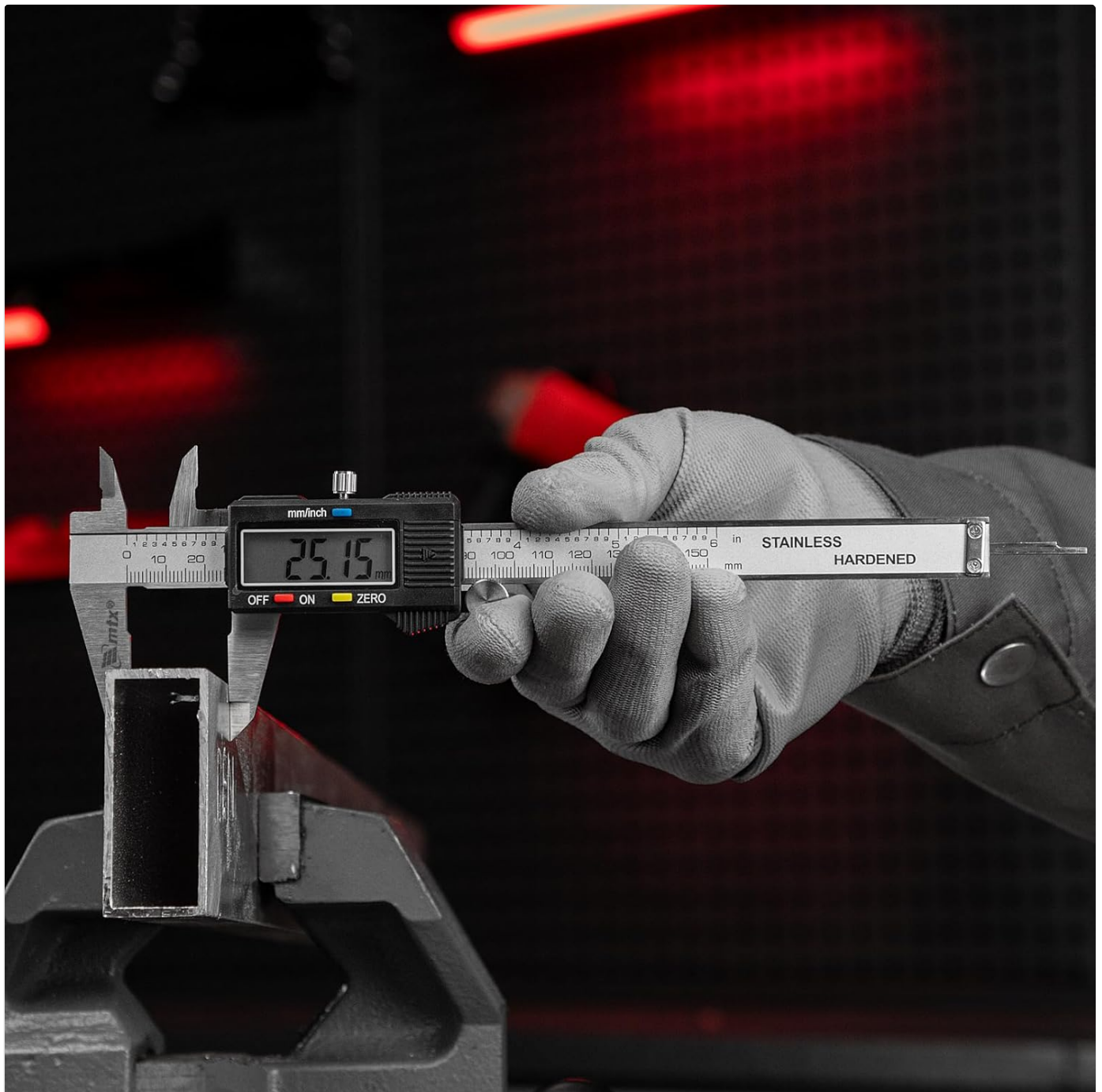
Image 5.2: Measuring the external dimension of a square tube.
