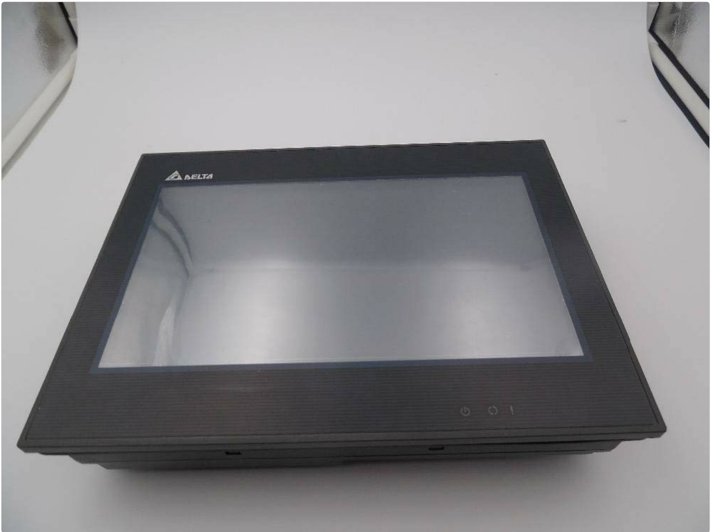
Figure 2.1: Front view of the GOWE Delta HMI DOP-B10E615 touch panel. The panel features a large display screen with the Delta logo at the top left and power/status indicators at the bottom right.
