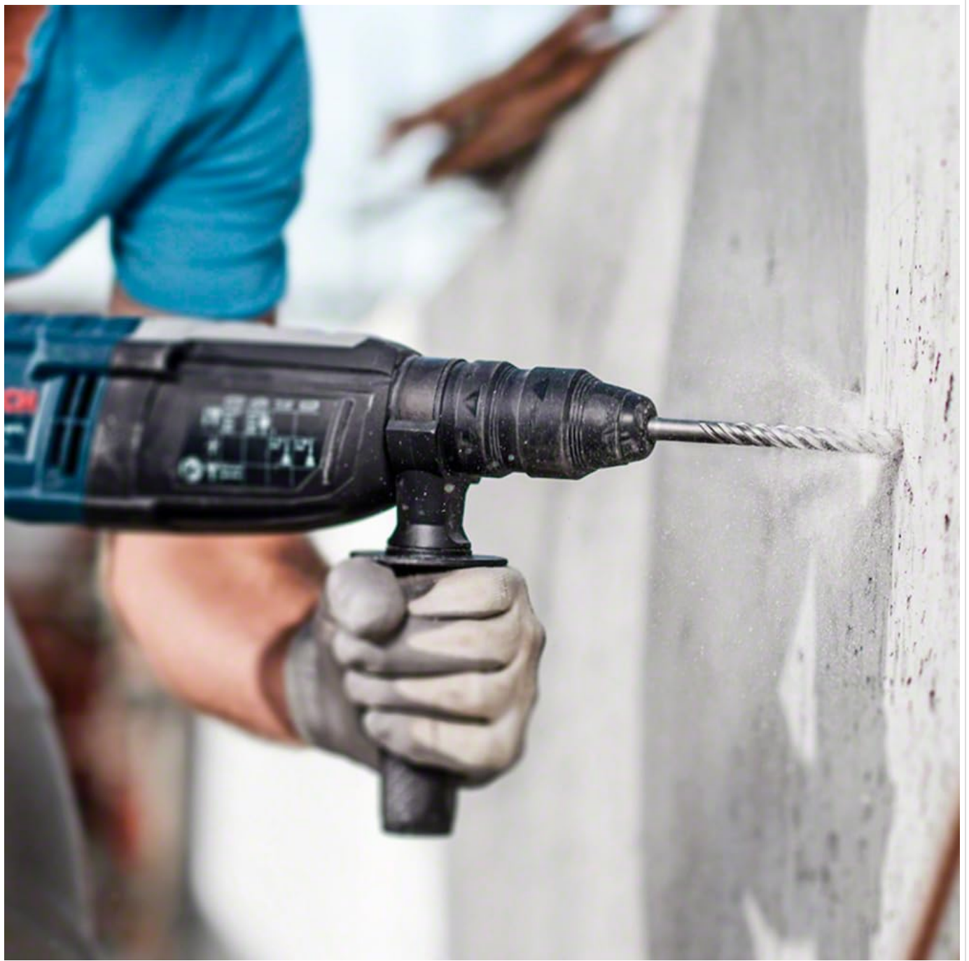
Figure 5: An operator using the Bosch GBH 2-28D Rotary Hammer Drill to create a hole in a concrete wall, demonstrating typical usage.
