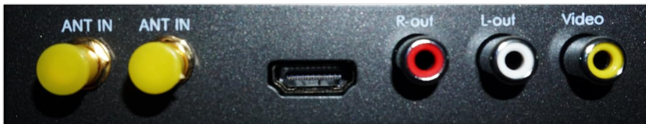
Figure 4: Close-up of the receiver's rear panel showing input/output ports. From left to right: two ANT IN (antenna) ports, HDMI output, R-out (right audio), L-out (left audio), and Video output.
