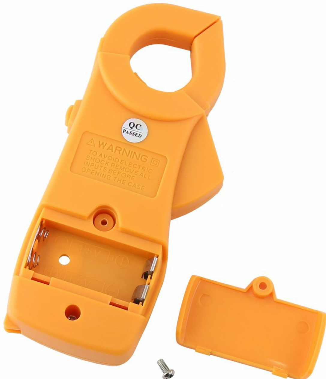
Figure 4.1: View of the battery compartment with the cover removed.
