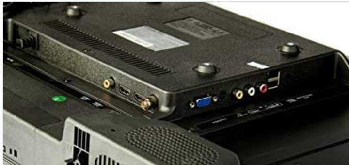
Rear view of the TV with ports including HDMI, USB, VGA, and RF antenna.
