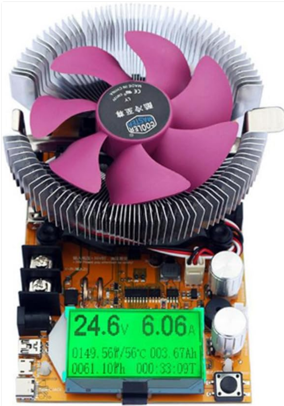
Figure 3: Close-up view of the LCD display, showing real-time voltage (V), current (A), temperature (°C), accumulated capacity (Ah), accumulated power (Wh), and elapsed time (T).
