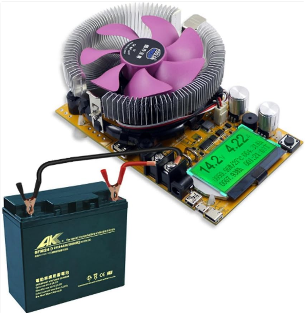
Figure 2: Example of the electronic load tester connected to a 12V battery using alligator clips on the screw terminals. This demonstrates a typical setup for discharging or testing a battery.
