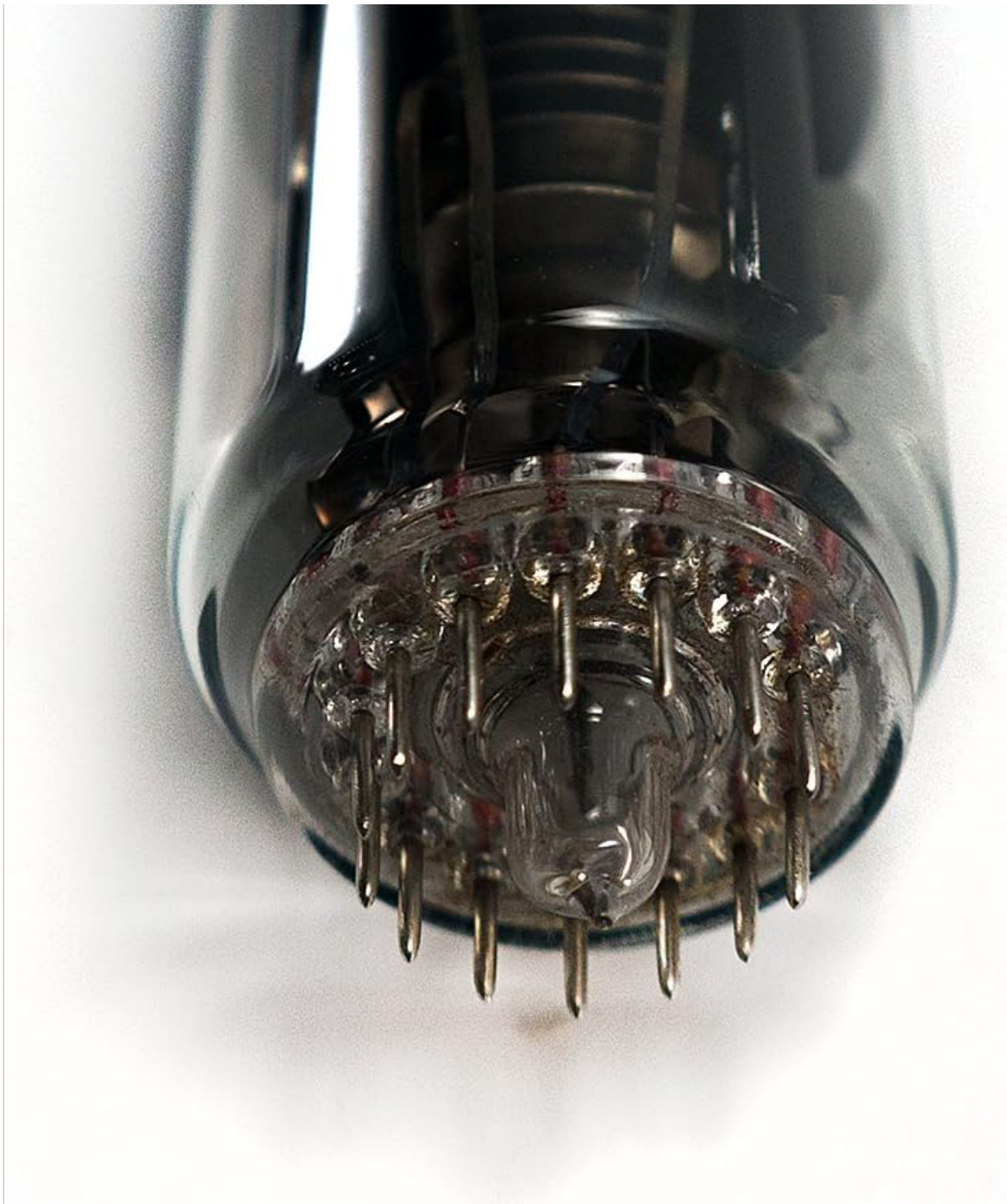
Figure 2.3: Close-up view of the 3LO11 Mini CRT's base pins, essential for electrical connections.
