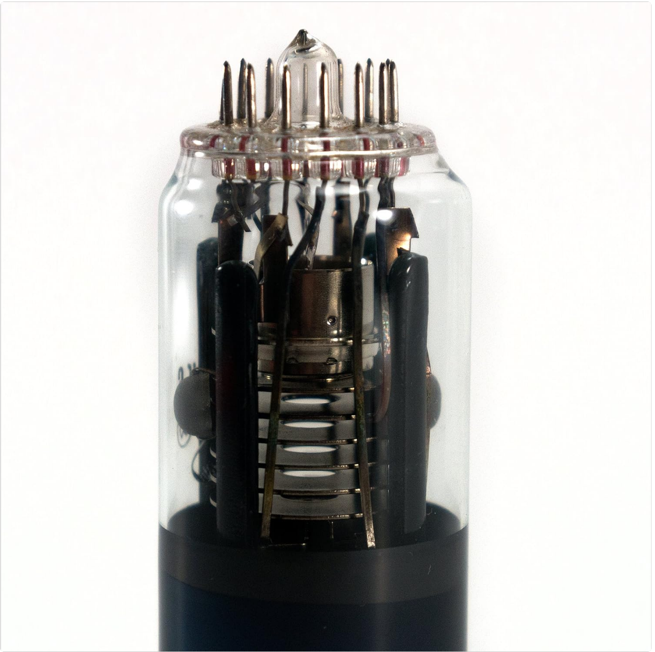
Figure 2.1: Side view of the 3LO1I Mini CRT, showing its glass envelope and internal components.
