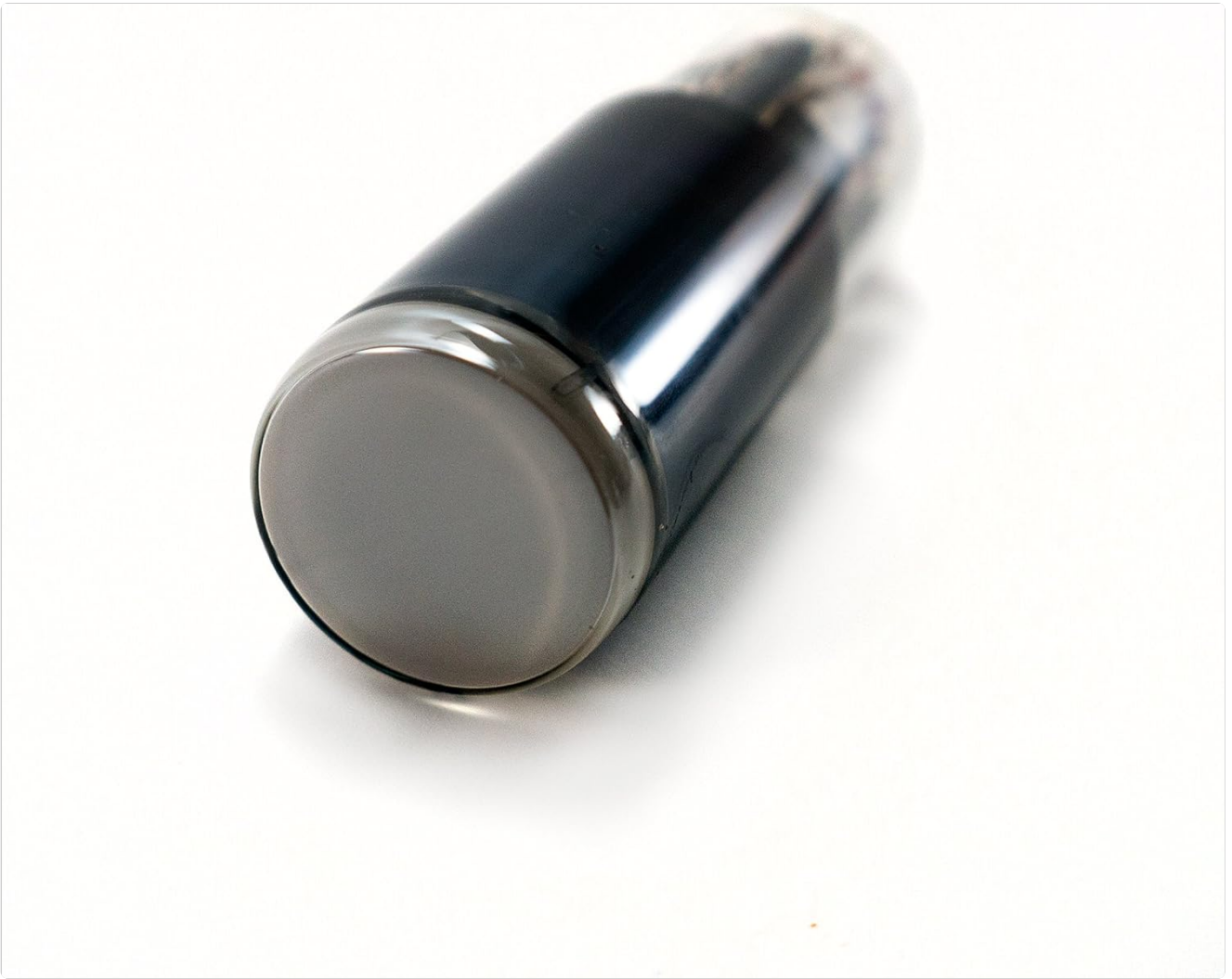
Figure 2.2: Angled view of the 3LO11 Mini CRT, highlighting the screen end and the base pins.
