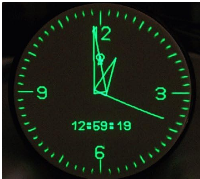
Figure 5.1: An example of a clock display on a green phosphor CRT, demonstrating the visual output capability.
