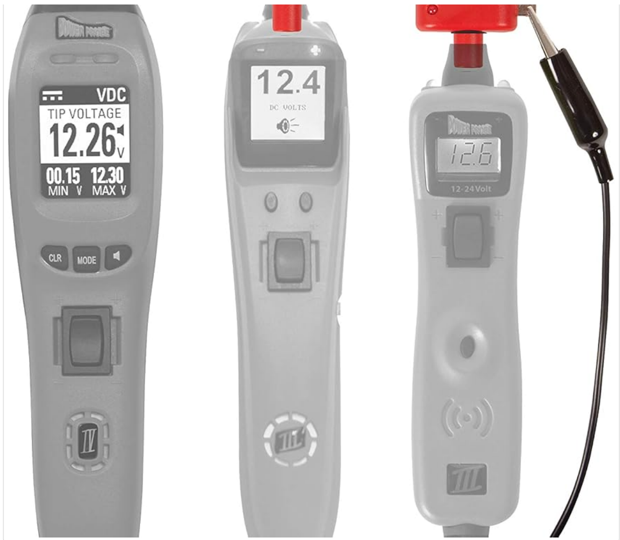
Image: The PPT5VA adapter shown connected to different models of Power Probe circuit testers, demonstrating its compatibility and connection method.
