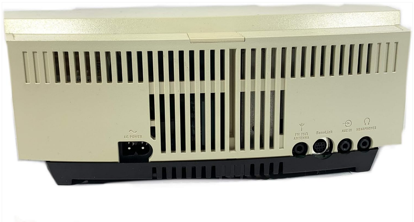
Image: Rear panel of the BOSE AWRCCC Wave Music System, illustrating the AC power input, FM antenna connection, BoseLink port, AUX IN, and Headphone jack.
