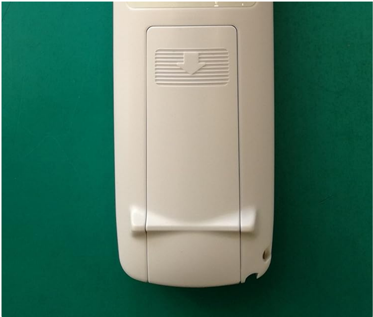
Figure 3: The rear view of the Sanyo RCS-6HVPUS4E remote control, showing the battery compartment and printed instructions for battery replacement and the reset button.
