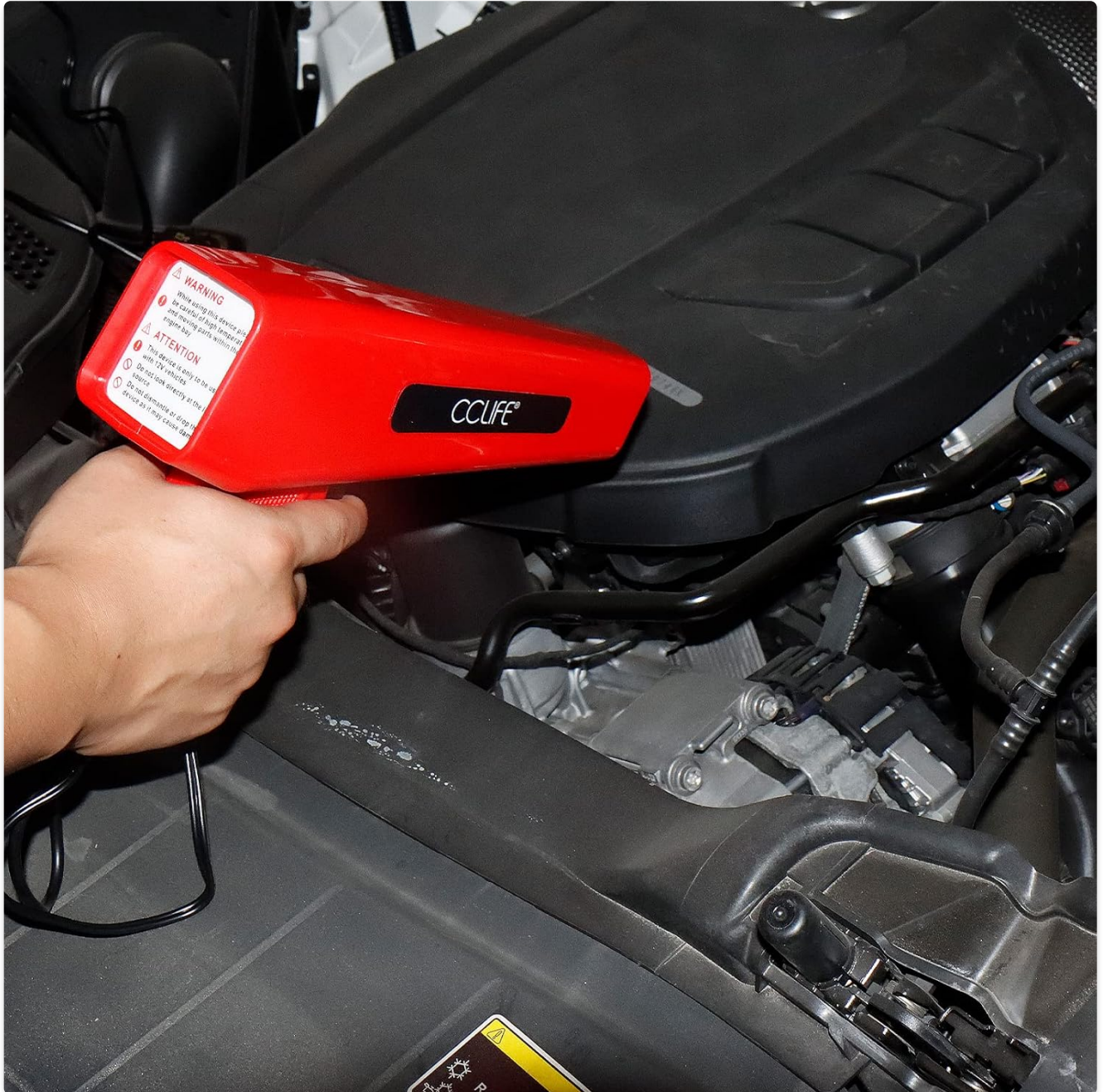
Image: A hand holding the red timing light, aiming it towards an engine's pulley system to check ignition timing.
