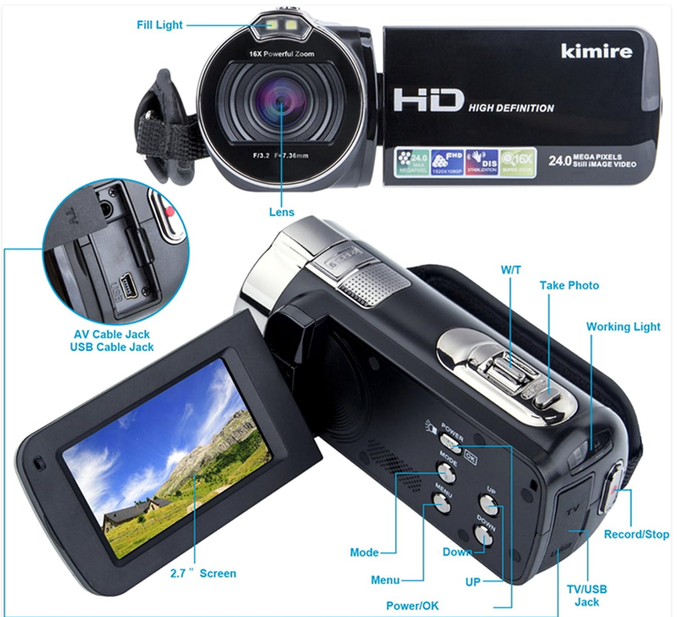
Figure 1: Front and side view of the camcorder with key components labeled. This includes the lens, fill light, 2.7-inch screen, AV cable jack, USB cable jack, W/T (Zoom) buttons, Take Photo button, Working Light, Record/Stop button, TV/USB Jack, Power/OK button, Menu button, and Up/Down navigation buttons.
