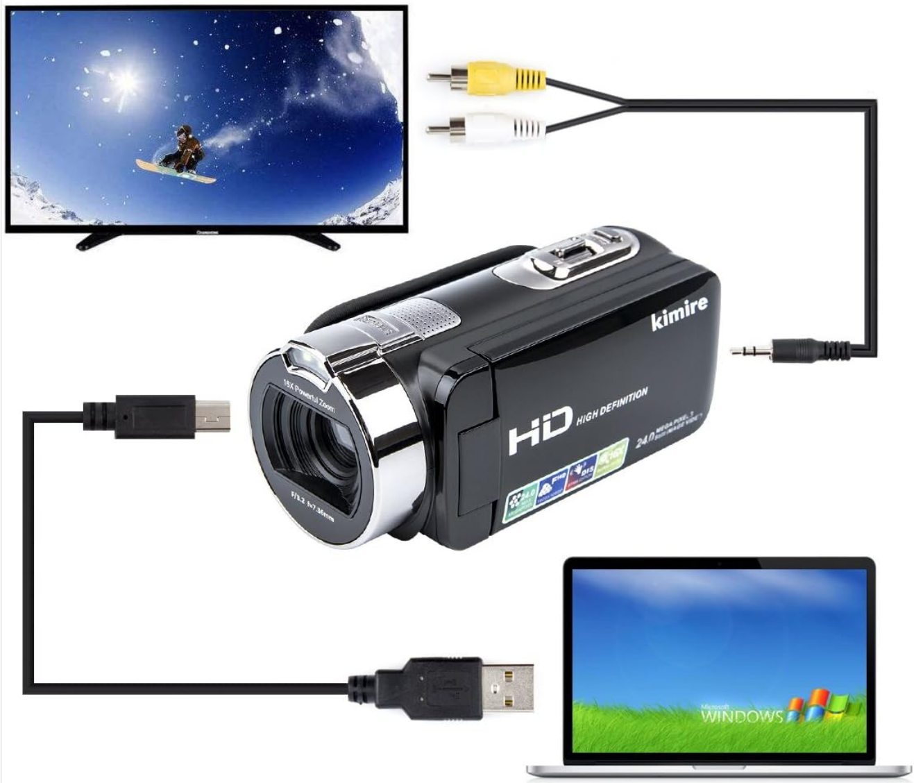
Figure 4: Illustration of connecting the camcorder to a television using the AV cable and to a computer using the USB cable.
