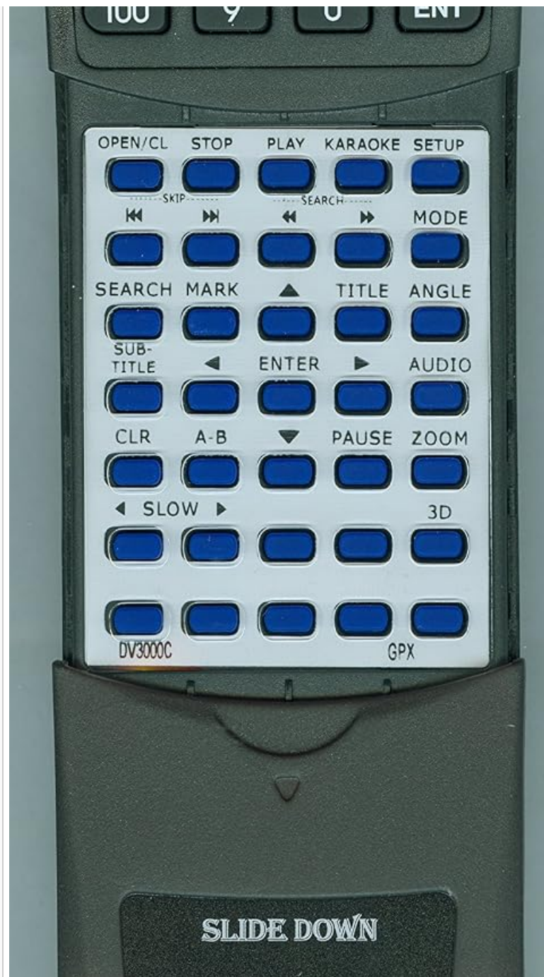
Figure 1: Front view of the Redi-Remote replacement remote for GPX DV3000C. The remote features a standard button layout for DVD player control, with a sliding cover revealing additional functions on the lower half.
