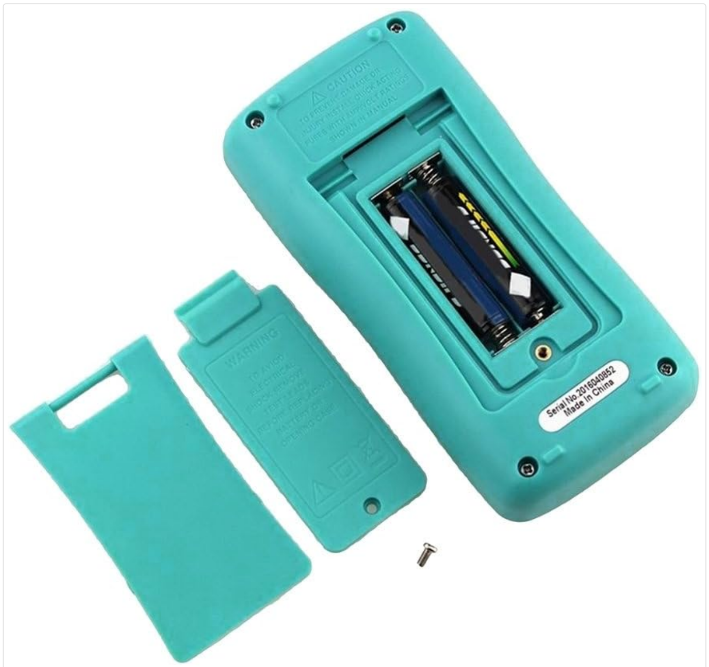
Figure 3: Rear view of the multimeter with the battery compartment open, showing the correct placement of AAA batteries.
