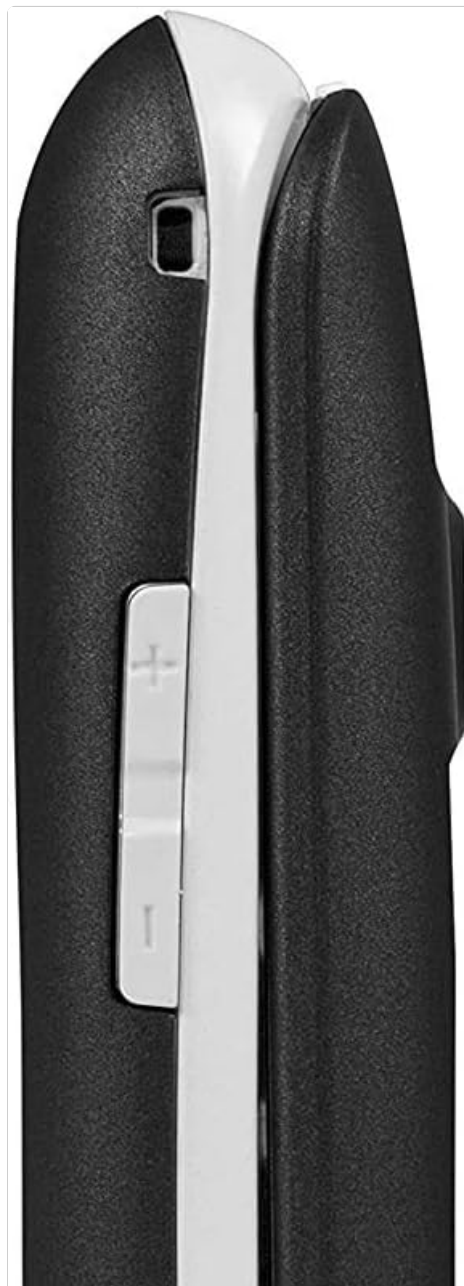
A side view of the Doro 2424, illustrating the 3.5mm headphone jack at the top and the volume up/down buttons on the side. These controls allow for easy adjustment of call and media volume.
