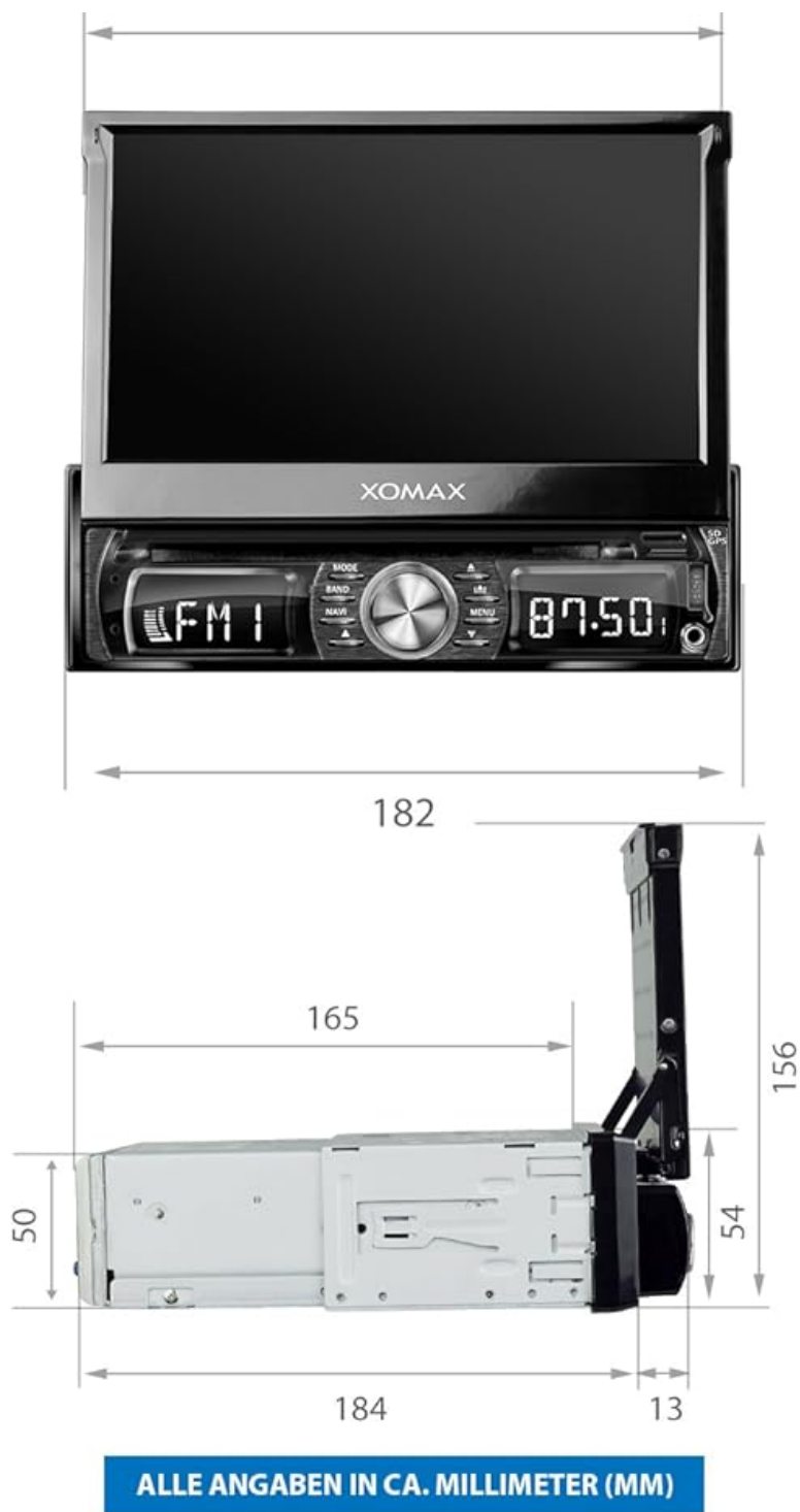
Image: Technical drawing displaying the dimensions of the XOMAX XM-DDA711 unit in millimeters, including width, height, and depth, both with the screen retracted and extended.
