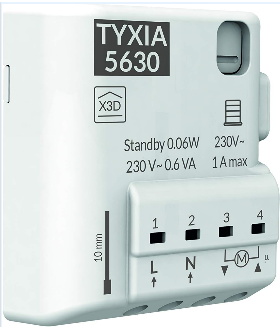
Image 2: Close-up view of the wiring terminals on the Delta Dore Tyxia 5630. Labels for Live (L), Neutral (N), and motor connections (M with up/down arrows) are visible, along with numbered terminals 1, 2, 3, and 4 for control inputs/outputs. Electrical specifications such as 'Standby 0.06W', '230V~', and '1 A max' are also indicated.
