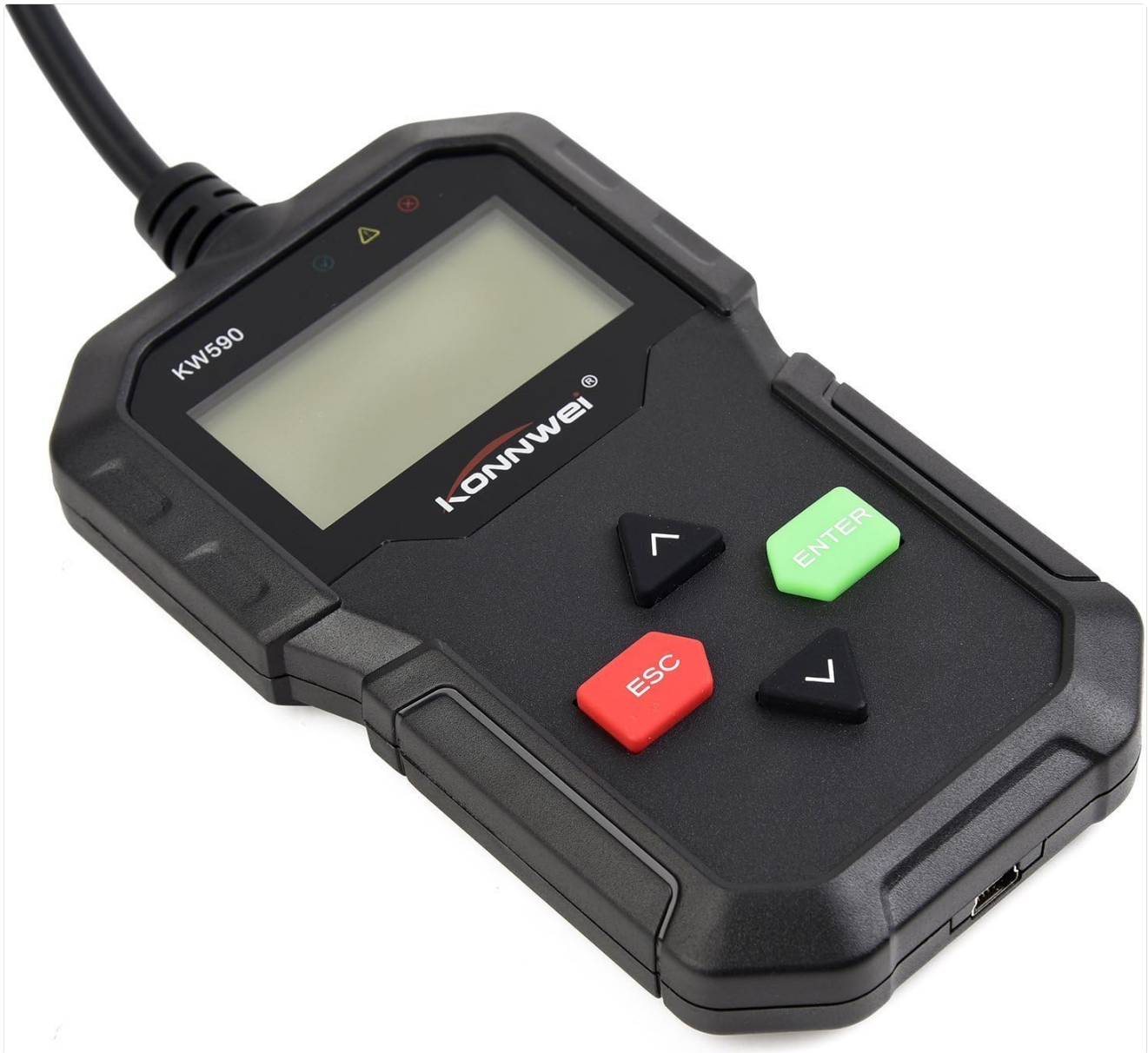
Figure 4.1: Front view of the KW590 scanner, highlighting the LCD display, ESC, ENTER, and navigation buttons.
