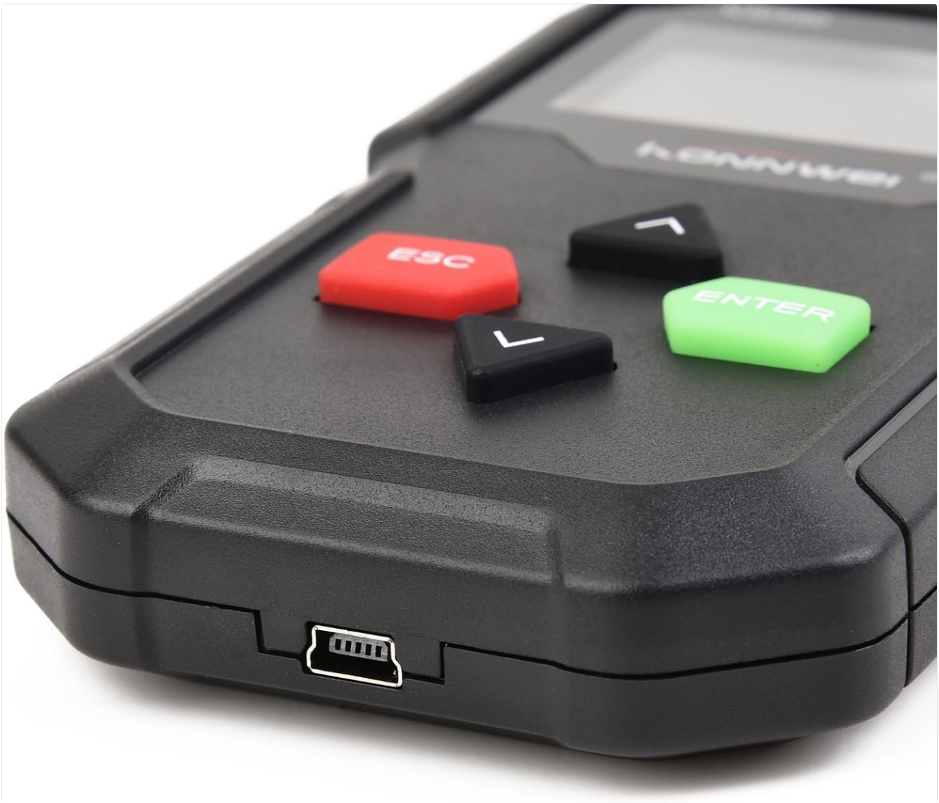
Figure 4.2: Side view of the KW590 scanner, showing the mini-USB port for PC connection.
