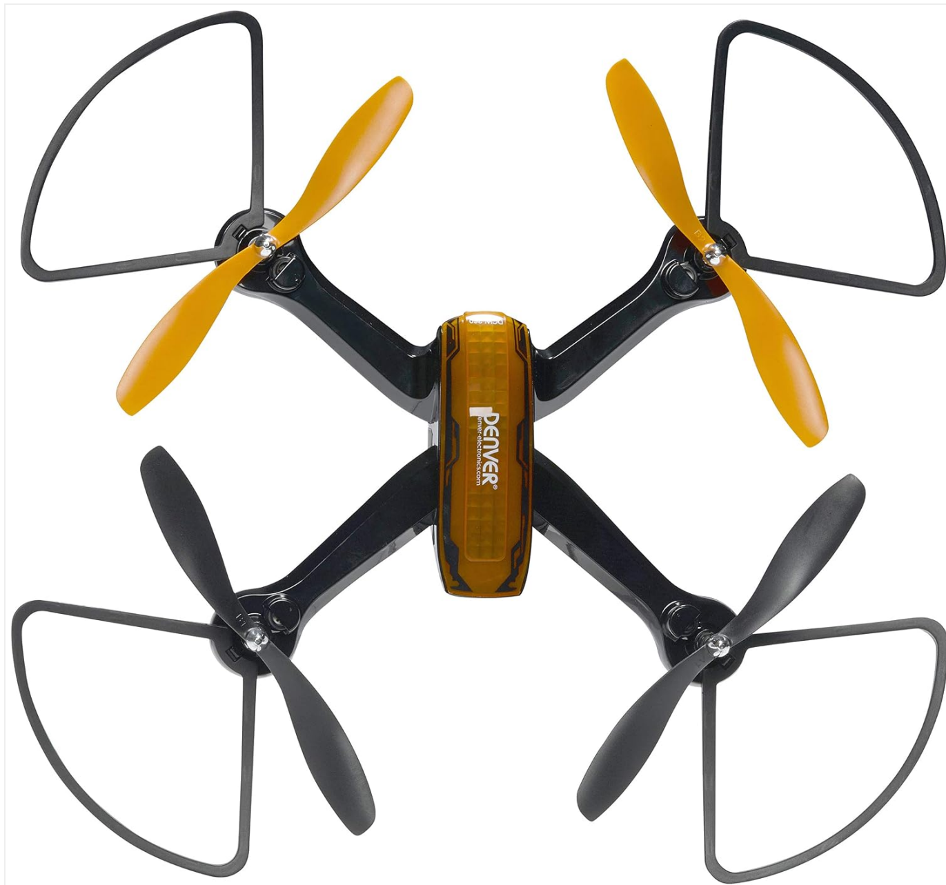
Figure 4.2: Top-down view of the Denver DCW-360 Drone. This perspective highlights the arrangement of the four propellers and their protective guards, along with the central body of the drone.
