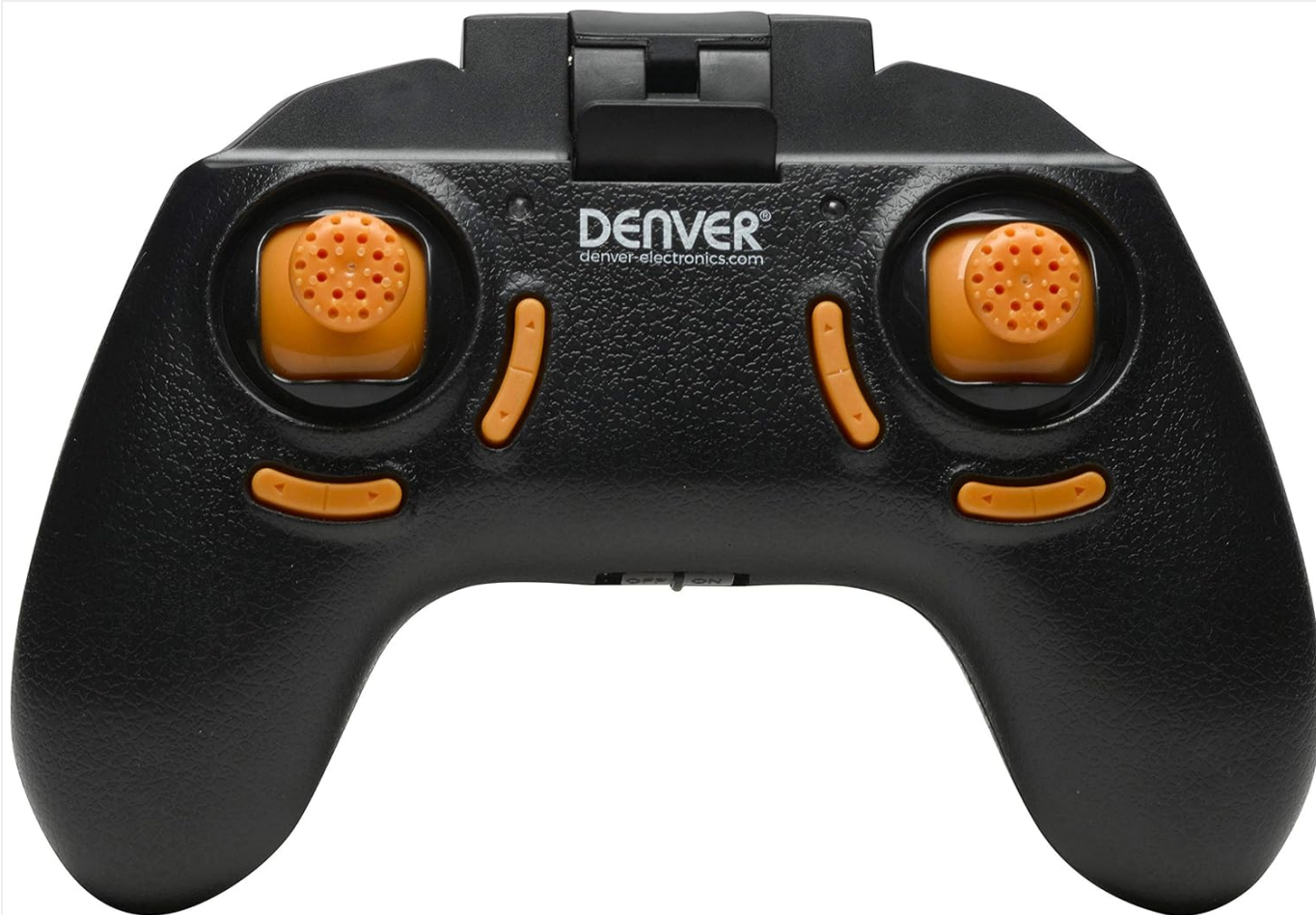
Figure 4.4: The remote controller for the Denver DCW-360 Drone. It features two joysticks, several control buttons, and a smartphone holder at the top.
