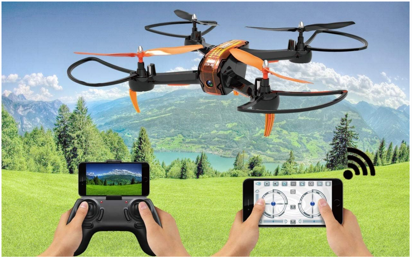
Figure 6.1: Illustration of the Denver DCW-360 Drone in flight, demonstrating control via both the physical remote controller and a smartphone app displaying the live video feed.
