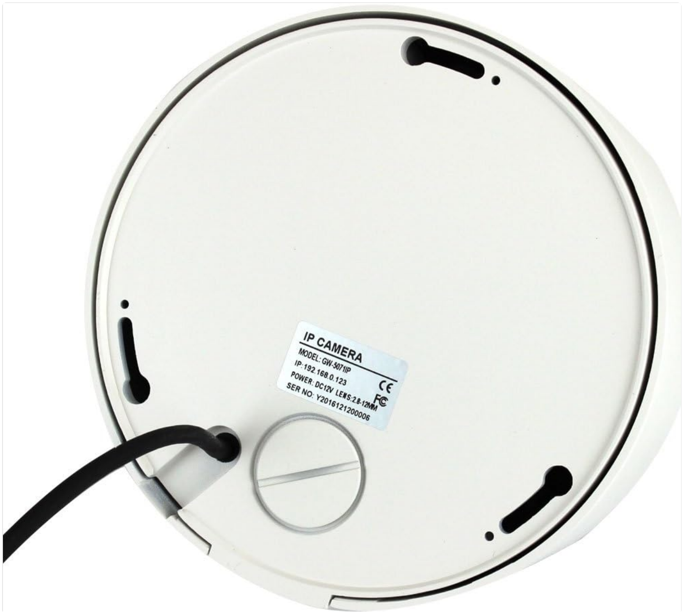
Figure 4.3: The bottom of the GW Security VD5071IP camera, displaying the model number (GW-5071IP), IP address, power requirements, and serial number. Mounting holes are also visible.
