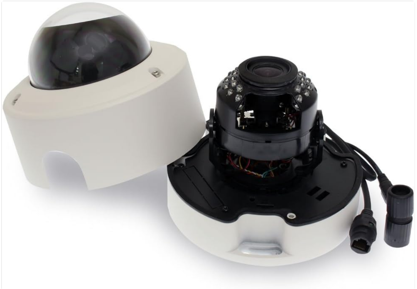
Figure 4.1: Internal view of the GW Security VD5071IP camera with its dome cover removed, revealing the lens, IR LEDs, and internal wiring. This image illustrates the camera's robust construction and key components.
