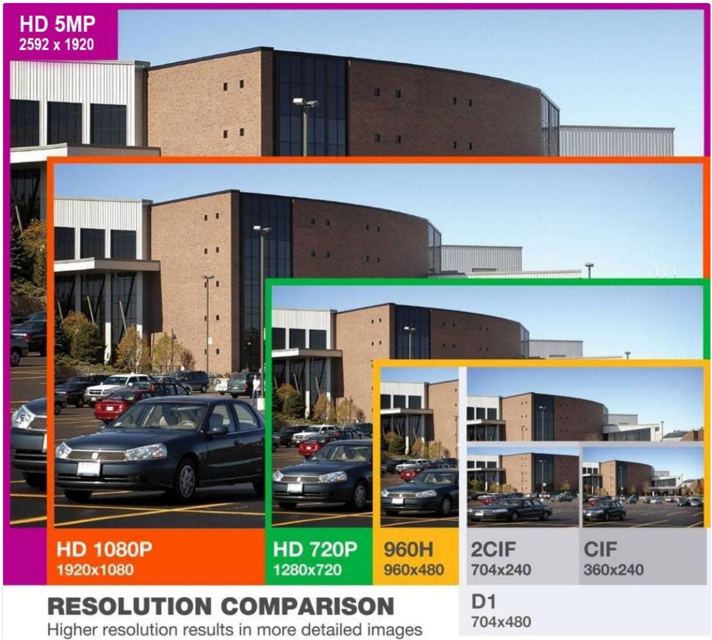
Figure 9.1: A visual comparison of different video resolutions, illustrating the superior detail provided by 5 Megapixel (2592x1920) compared to lower resolutions like 1080P (1920x1080) and 720P (1280x720).
