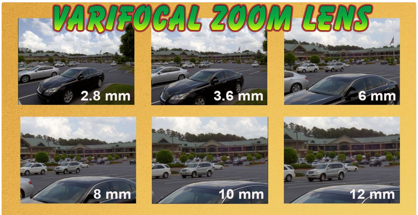
Figure 6.2: A visual comparison demonstrating the effect of adjusting the varifocal lens from 2.8mm (wide angle) to 12mm (narrower, zoomed-in view). This illustrates how the field of view changes with different focal lengths.
