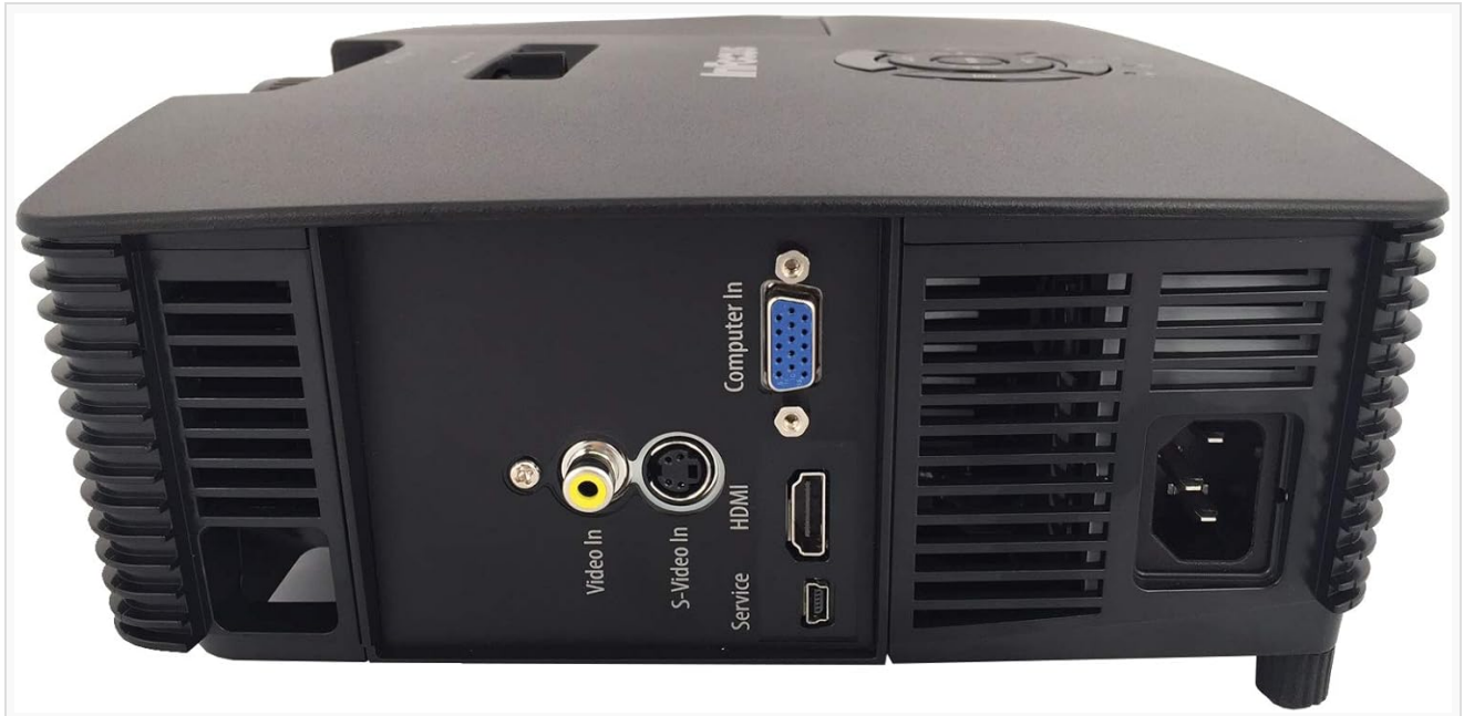
Image 3.3: Rear view of the InFocus IN112XV projector. This image displays the available connection ports, including Video In, S-Video In, Computer In (VGA), HDMI, and the power input.
