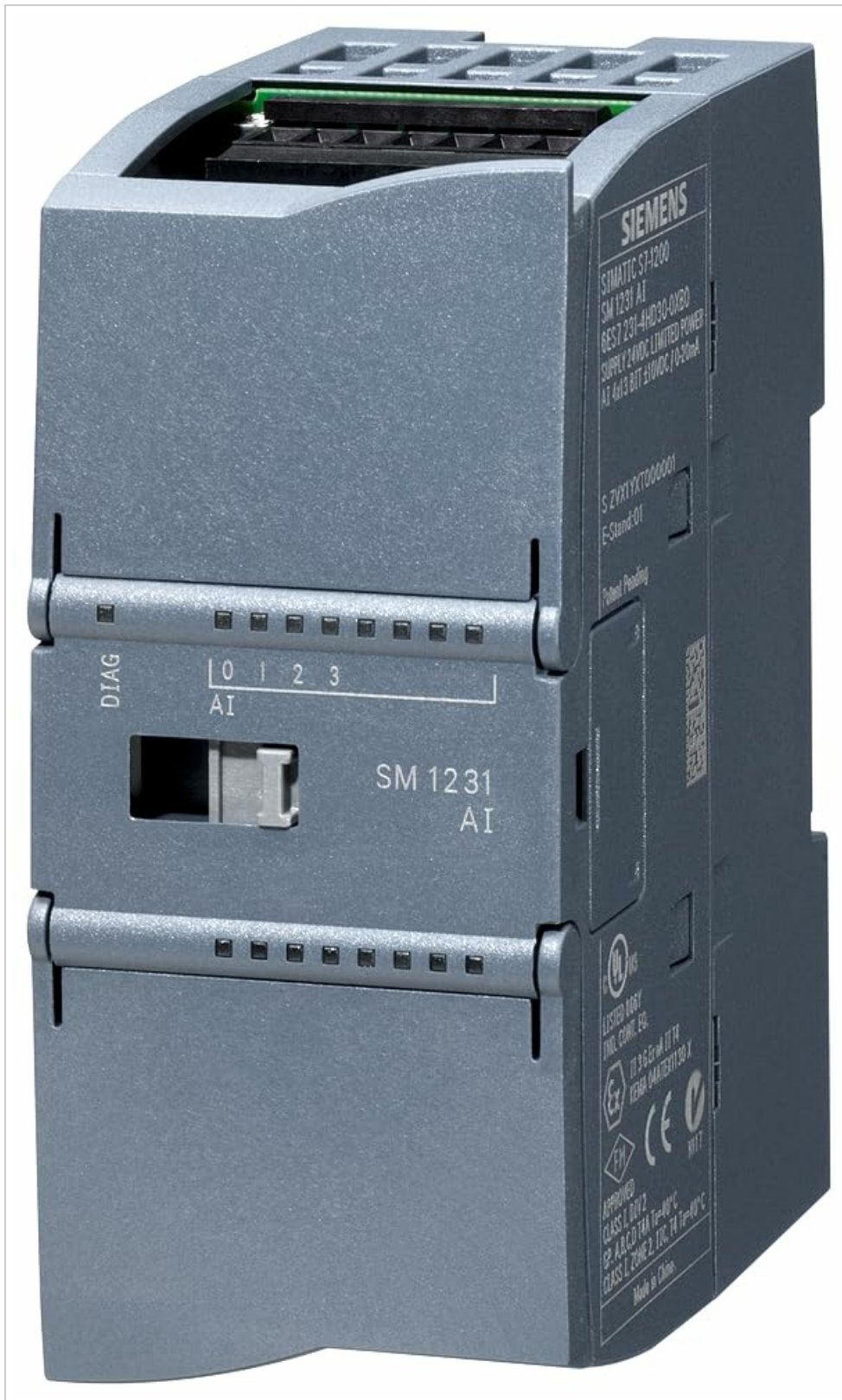
Figure 1: Siemens SIMATIC S7-1200 SM 1231 RTD Analog Input Module. This image displays the front view of the gray-colored module, featuring the Siemens logo and 'SIMATIC S7-1200 SM 1231 AI' labeling on the right side. The center section shows a 'DIAG' indicator, input terminals labeled '0', '1', '2', '3' for AI, and a sliding switch. The bottom section includes regulatory markings and certifications.
