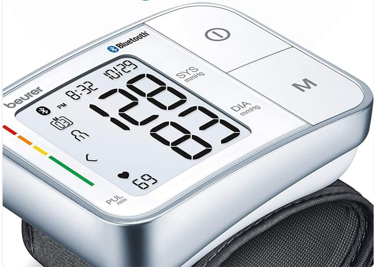
Figure 5: The resting indicator helps ensure you are calm and sitting correctly for accurate readings.
