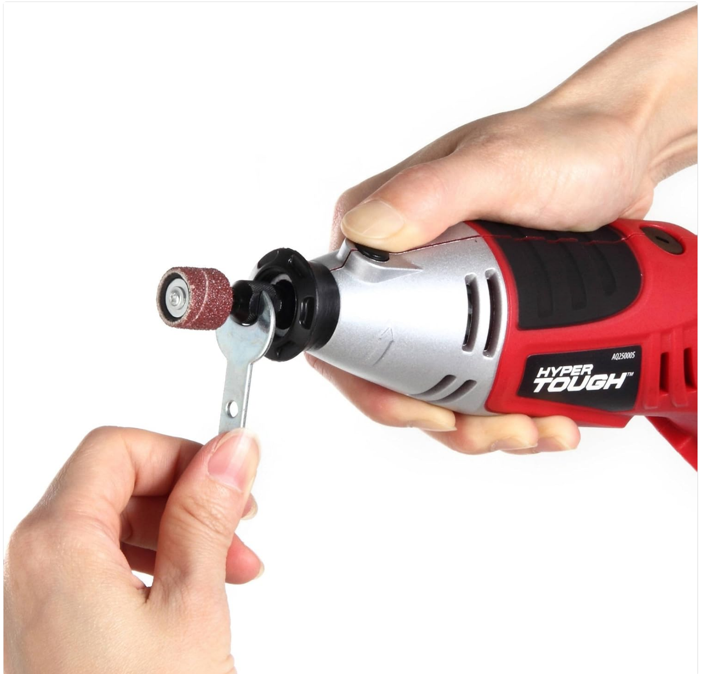
Figure 4.1: Illustration of attaching an accessory bit to the rotary tool. Ensure the tool is unplugged before changing bits.
