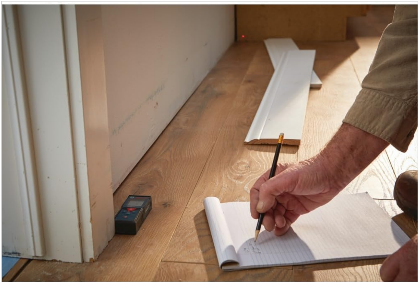
Figure 2: A user positioning the Bosch GLM165-40 laser measure against a wall to take a distance measurement.
