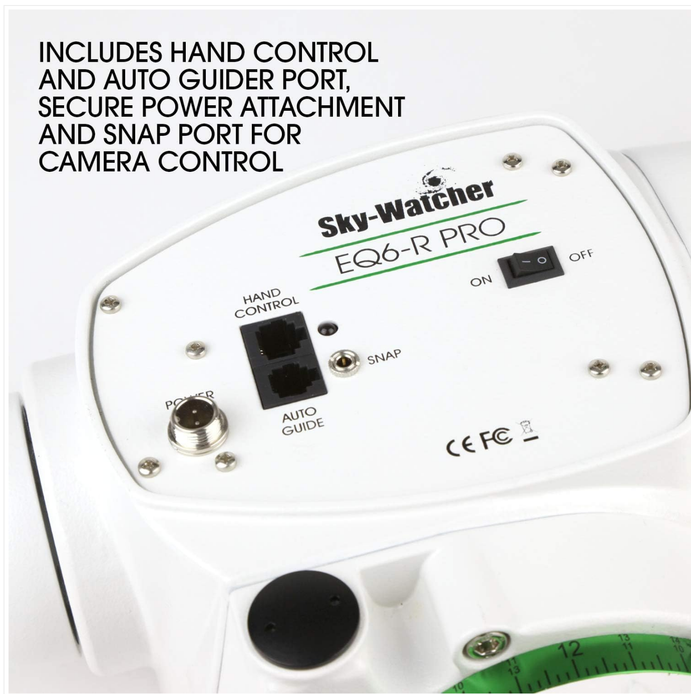
Image: Close-up view of the Sky-Watcher EQ6-R Pro mount's control panel, showing the Hand Control, Auto Guide, Snap, and Power ports. These ports allow for connection of the SynScan hand controller, an autoguider for precise tracking, a DSLR camera for remote shutter control, and the main power input.
