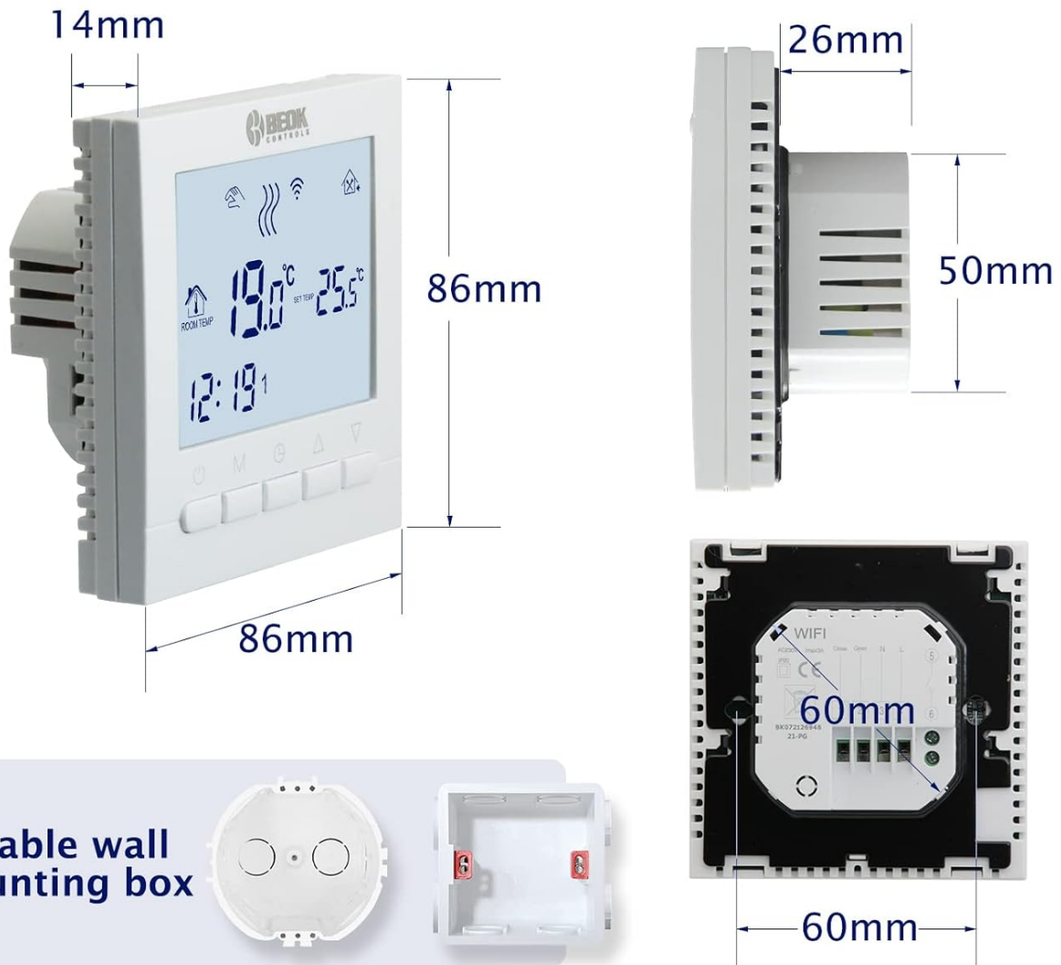
Image 3.3: Dimensions of the thermostat unit (86mm x 86mm front, 50mm depth) and a suitable wall mounting box (60mm x 60mm).
