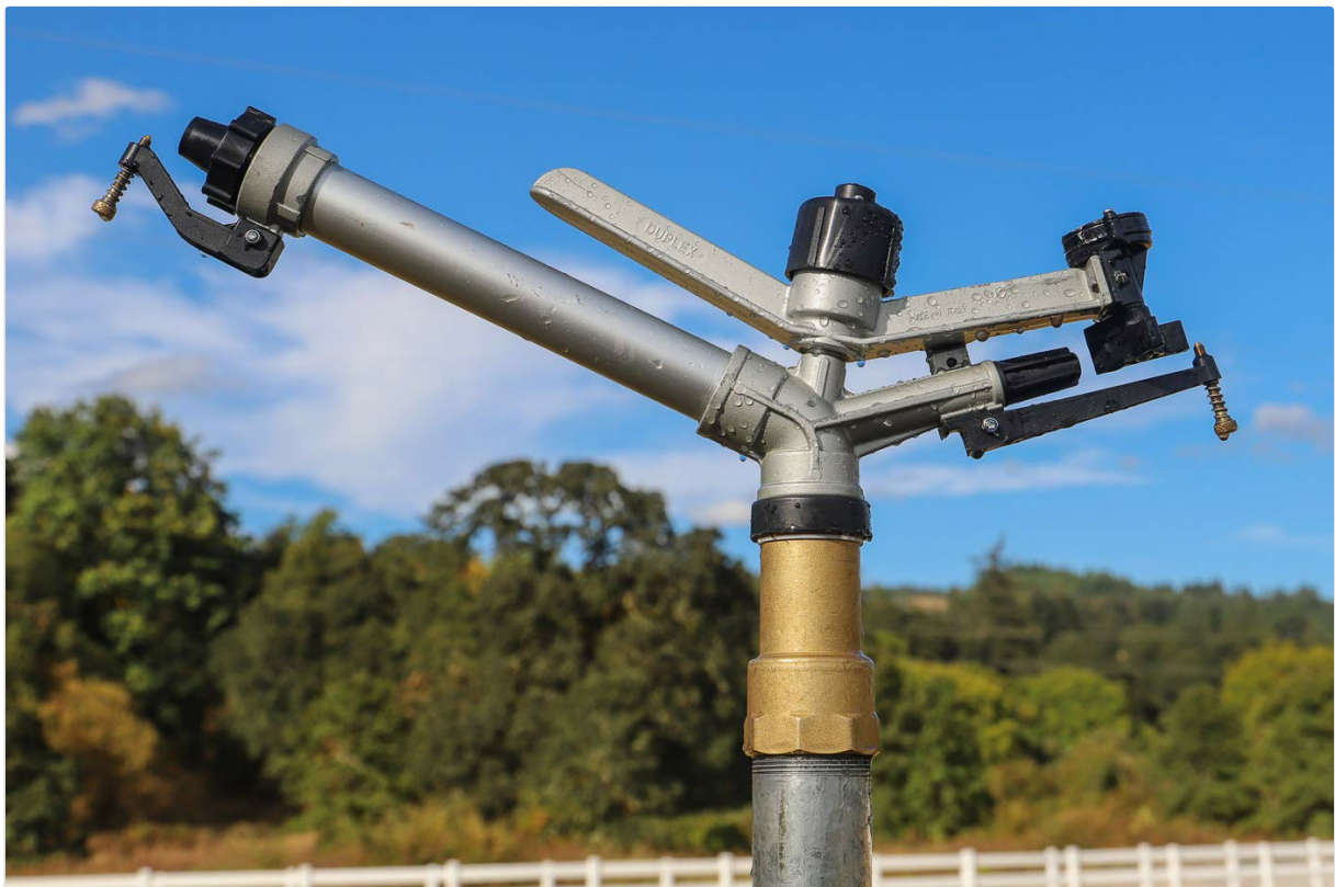
Figure 2: The Sime Duplex sprinkler installed on a riser, ready for operation. Proper vertical mounting is crucial for even water distribution.
