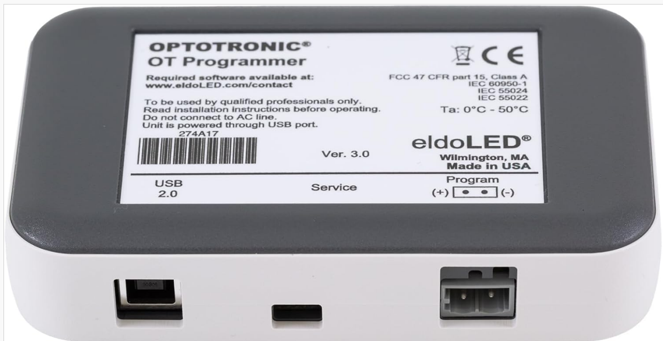
Image 3.1: Top view of the eldoLED Optotronic OT Programmer, highlighting the USB 2.0 port and the Program (+)/(-) interface.
