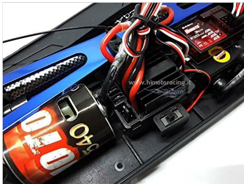
Image 3.4: Detailed view of the RC-540 brushed motor and associated electronics.
