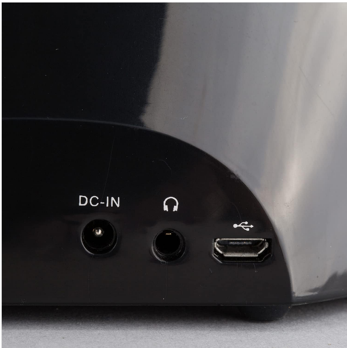
Image: Rear view of the Sungale KWS433+-3, showing the DC-IN port, headphone jack, and USB port.
