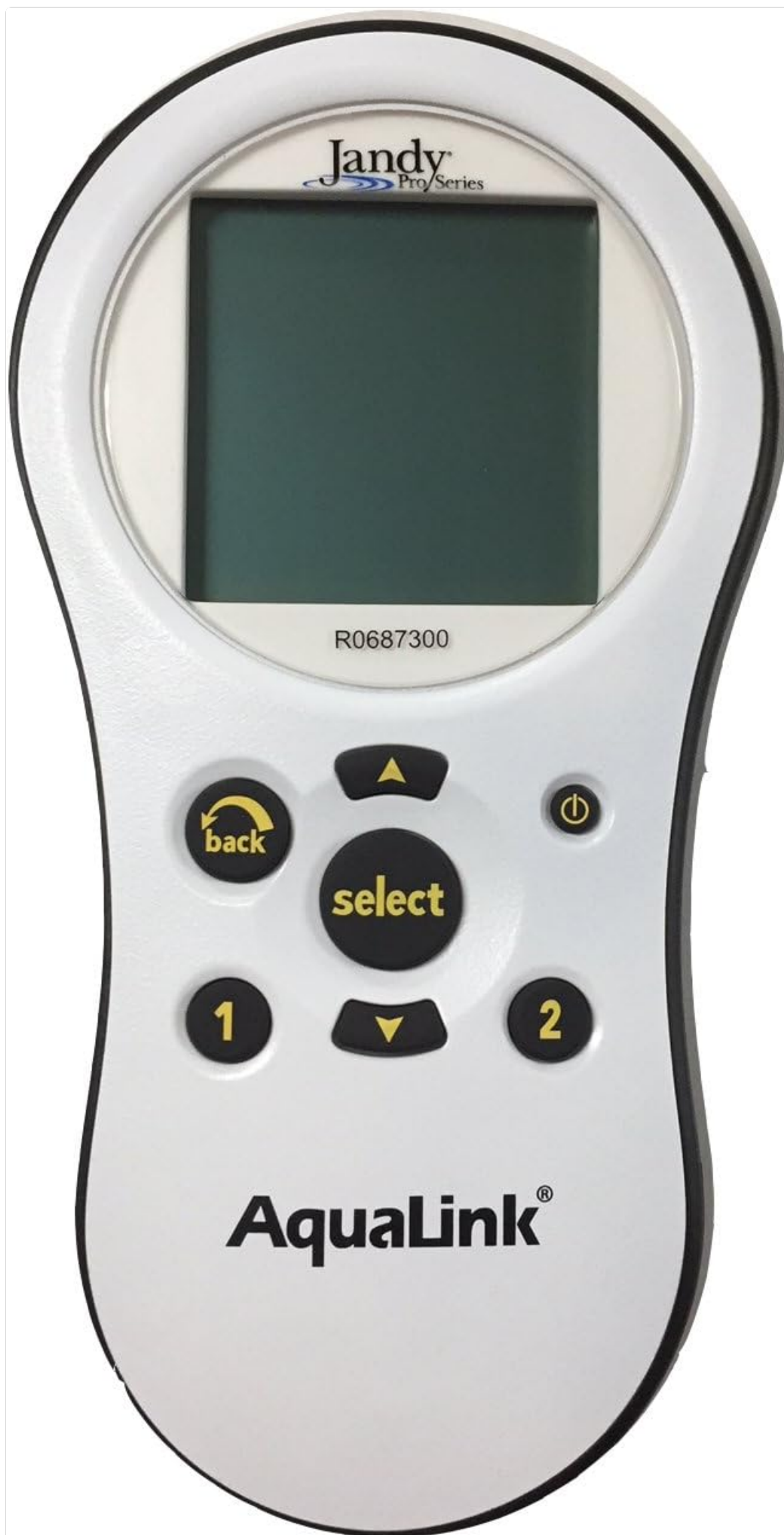
Figure 1: Front view of the AquaPalm Wireless Remote, showing the display, navigation buttons (back, up, down, select), power
