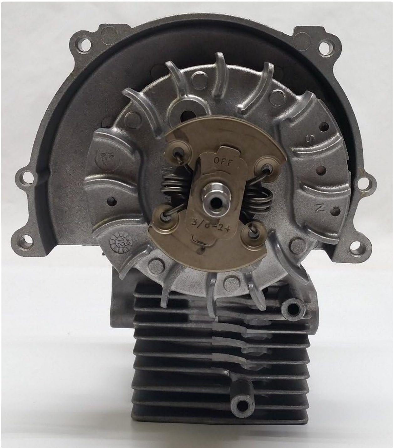
Figure 3: Front view of the short block, highlighting the flywheel and clutch mechanism, which connects to the trimmer's drive shaft.
