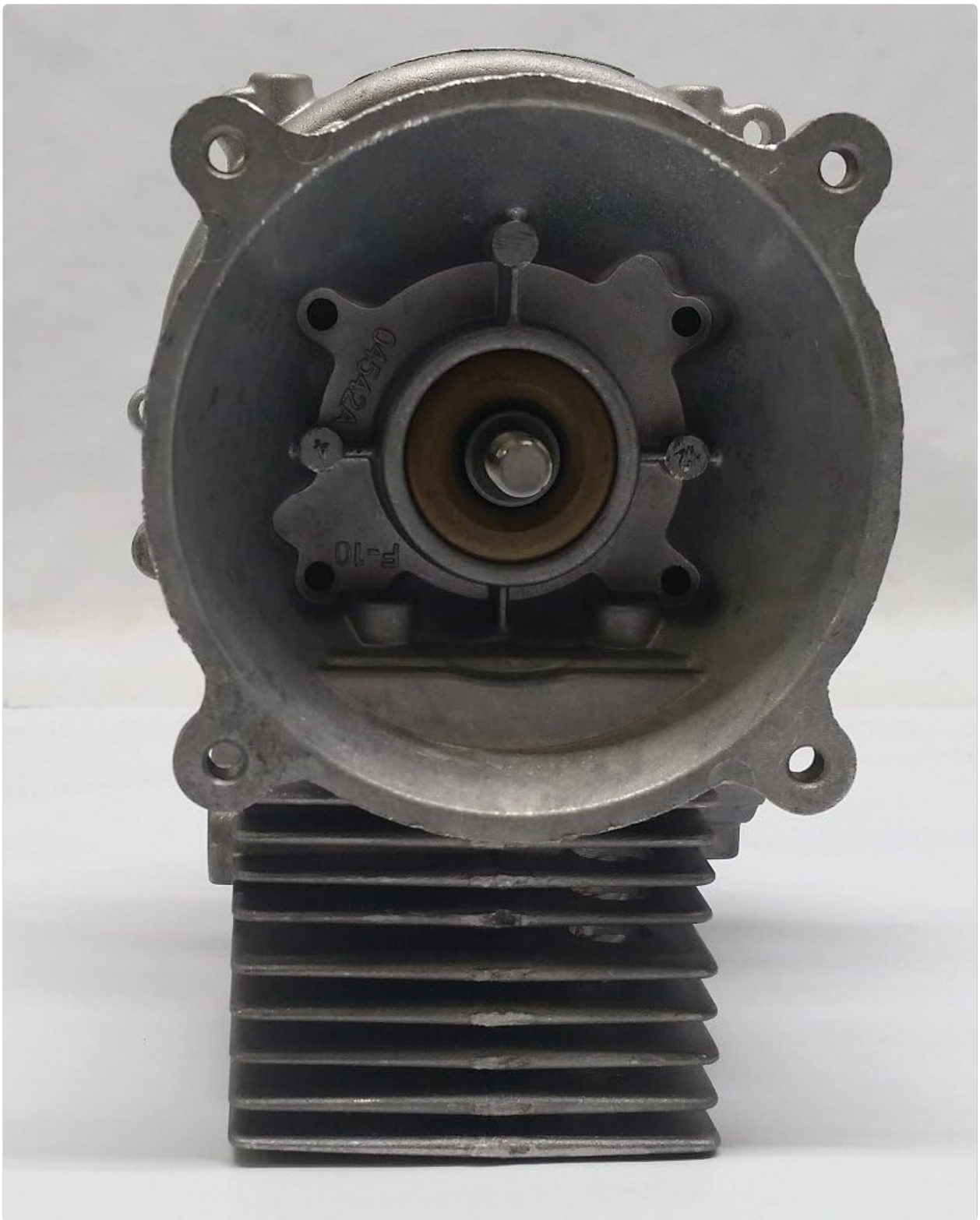
Figure 4: Rear view of the short block, illustrating the intake manifold area where the carburetor would typically attach.
