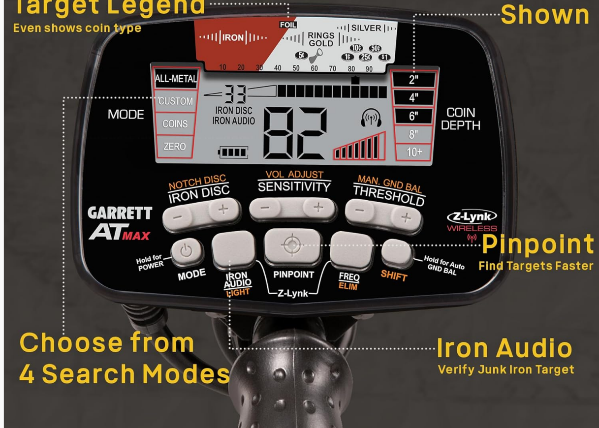
Figure 3: The AT Max control panel displays target ID, depth, and allows selection of various search modes and settings.
