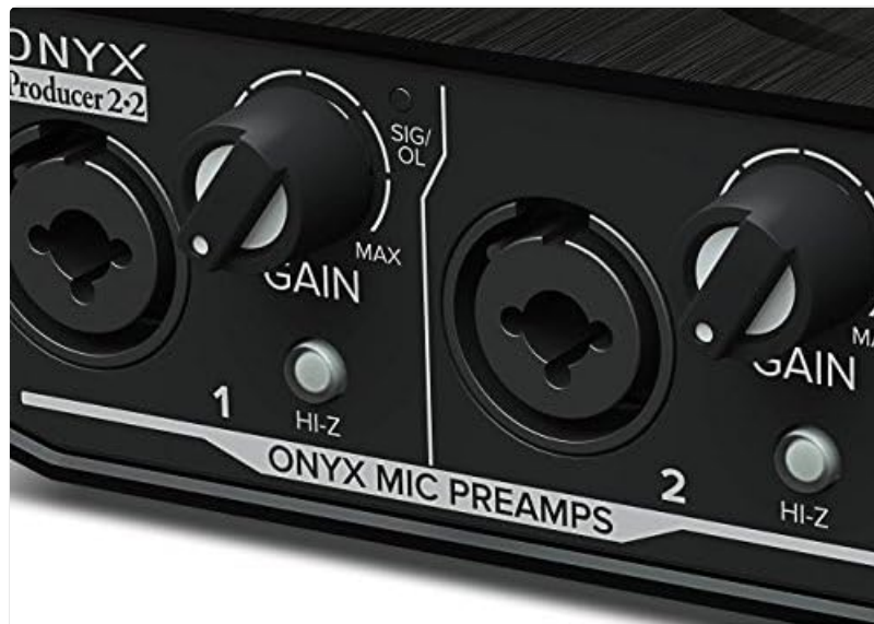
Figure 4: Close-up view of the Onyx mic preamps and gain controls.
