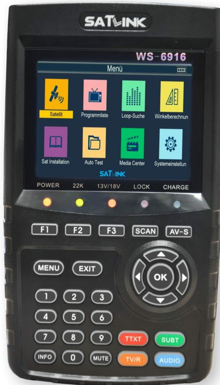
Figure 4.1: Front view of the SATLINK WS 6916 Digital Satellite Meter. This image shows the 3.5-inch TFT LCD screen and the main control buttons for navigation and function selection.
