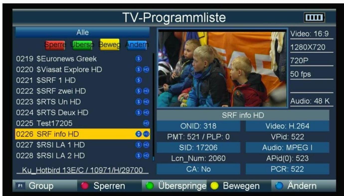
Figure 6.3: TV Program List Screen. The TV Program List allows users to browse available channels and view their technical specifications such as video resolution and audio format.
