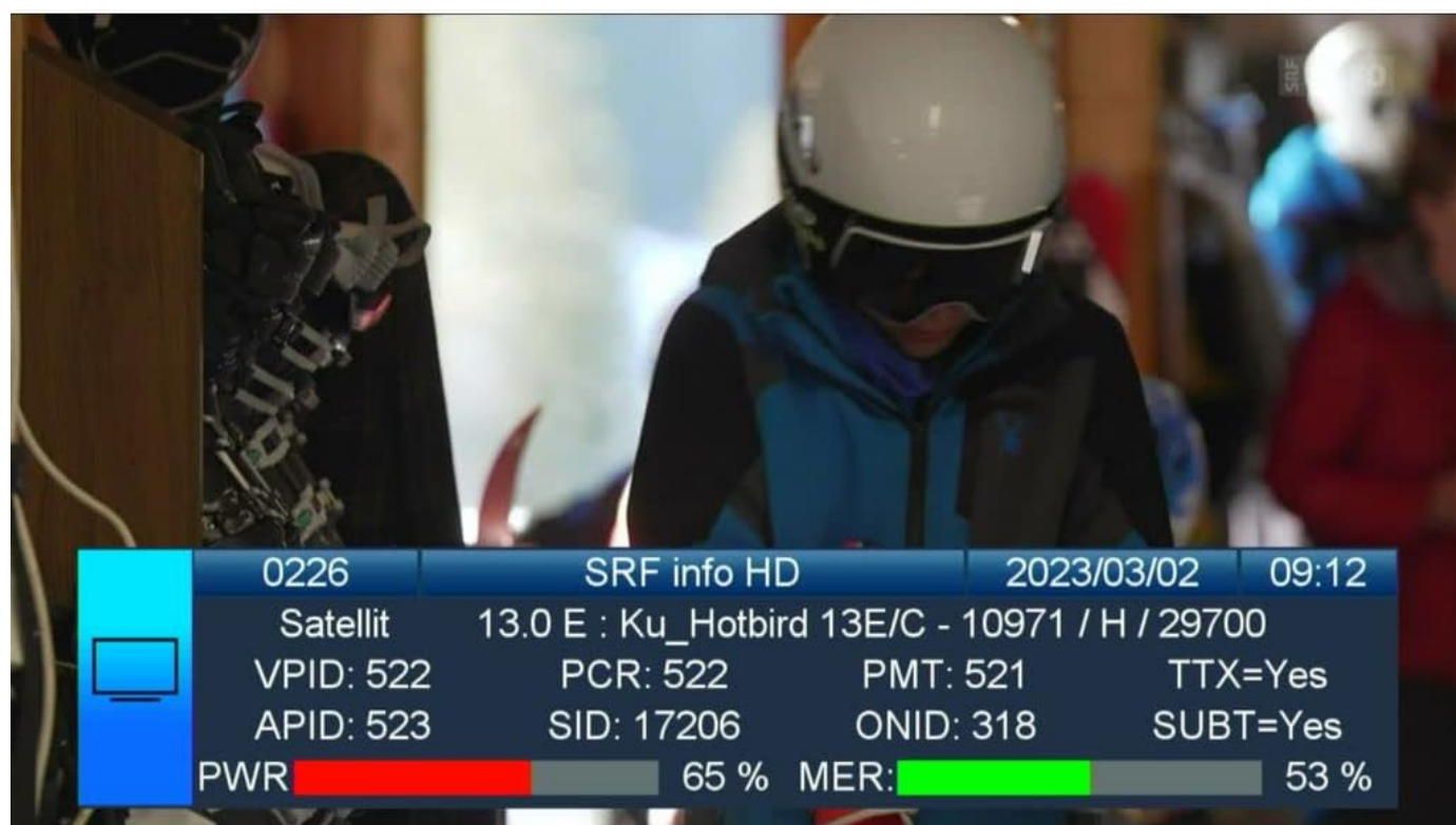
Figure 6.4: Live TV Preview Screen. The device can display live television channels, providing visual confirmation of signal quality along with detailed channel parameters.
