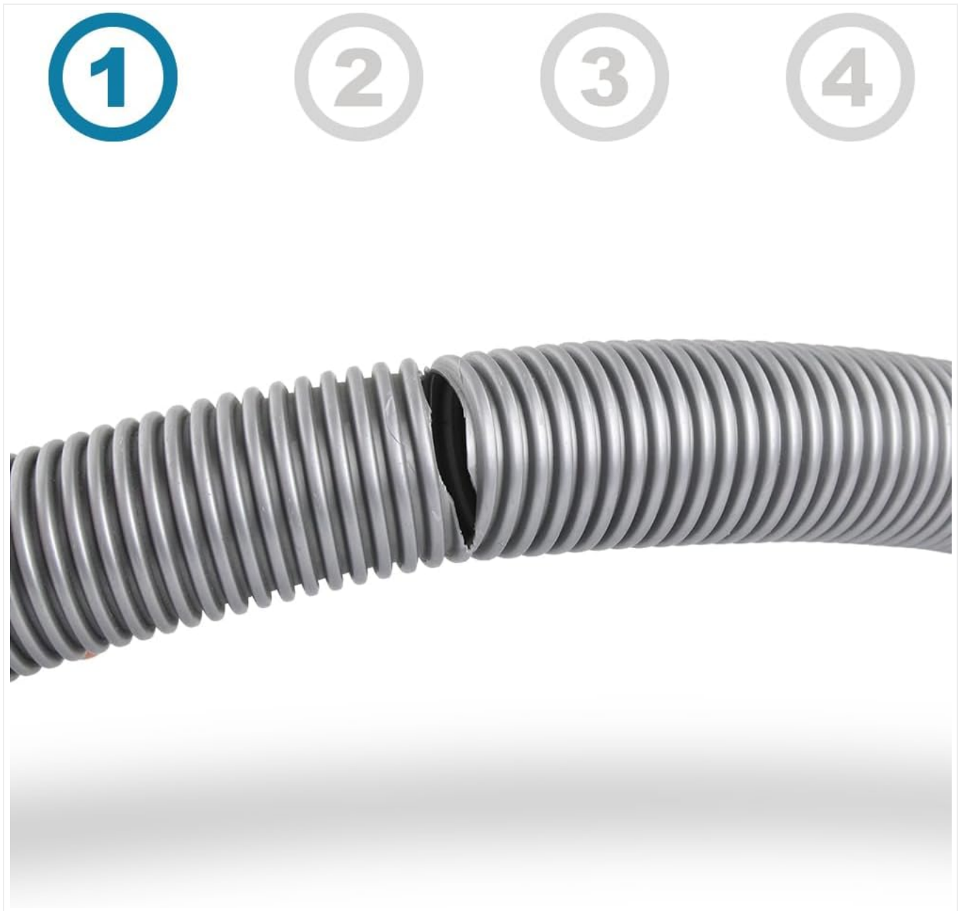
Figure 1: A vacuum cleaner hose with a visible tear, indicating the area requiring repair.
