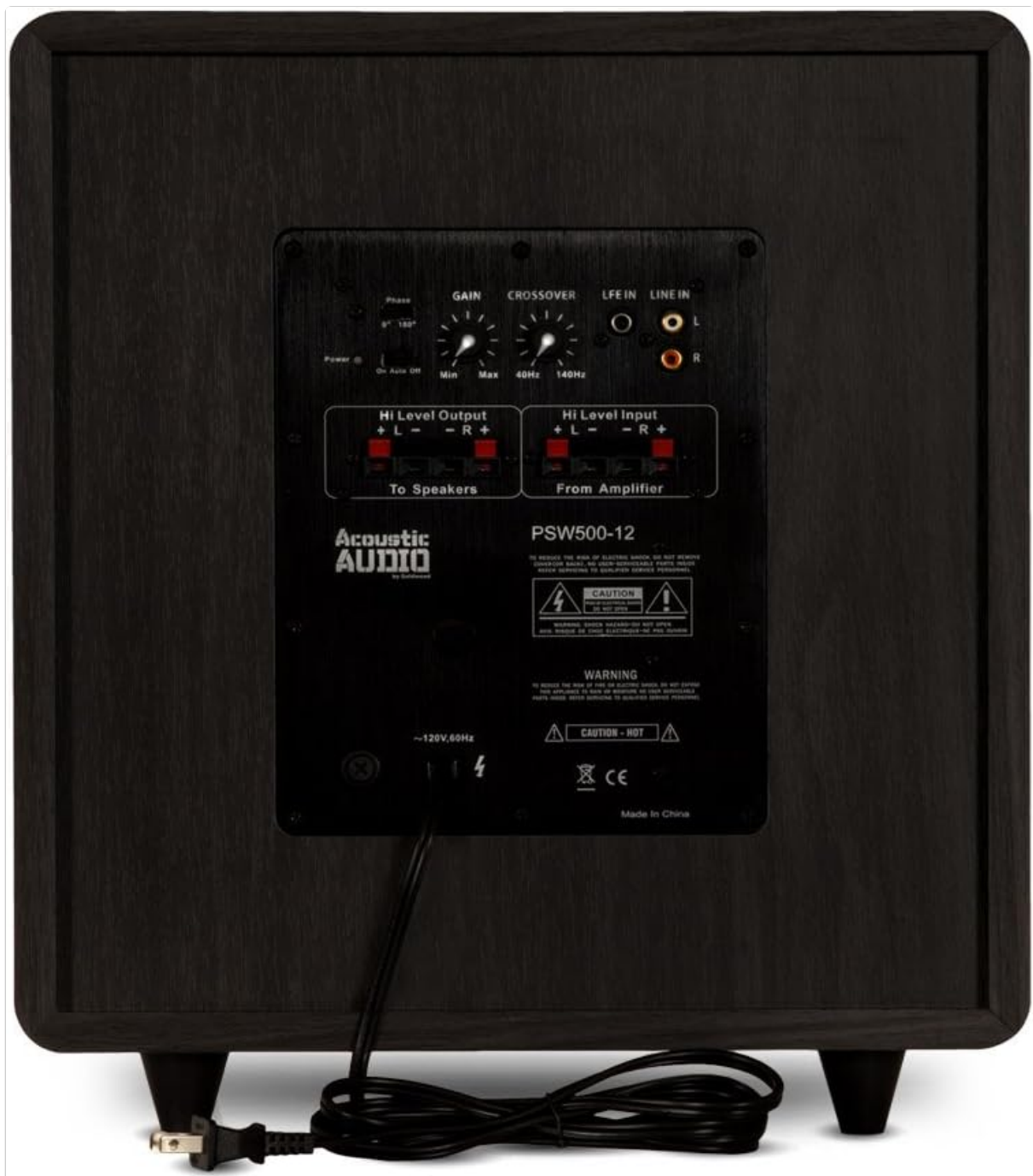
Image: Rear panel of the subwoofer displaying the power switch, power input, LFE/Line inputs, High Level inputs/outputs, Phase control, Gain control, and Crossover frequency control.
