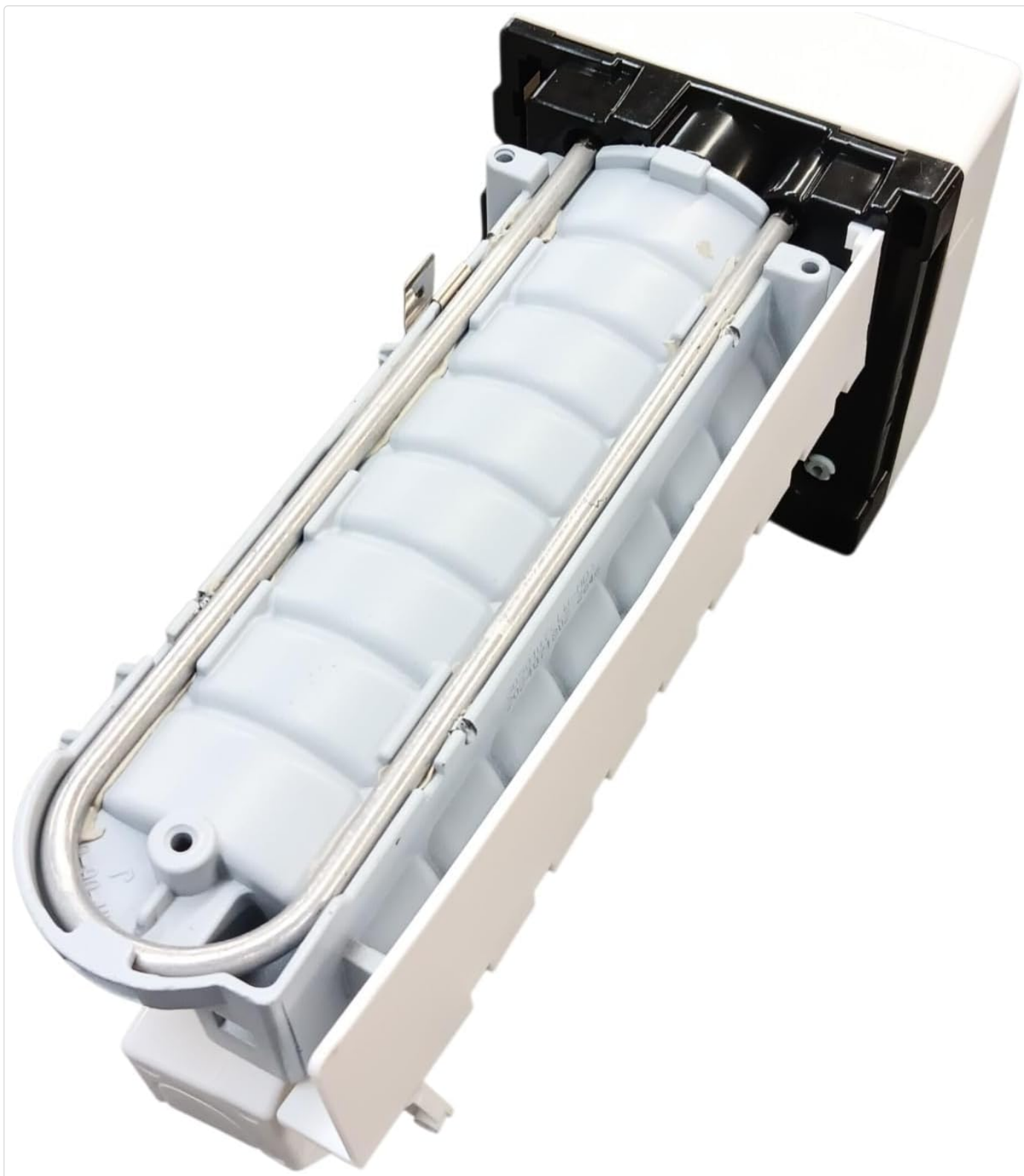
Image 6.1: Bottom view of the icemaker, revealing the ice mold where water freezes and the heating element that aids in releasing ice cubes.
