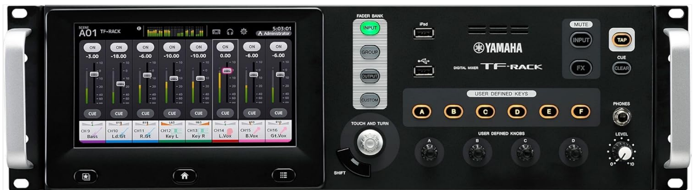
Figure 5.1: Front panel of the Yamaha TF-Rack, highlighting the large touchscreen display, FADER BANK buttons, USER DEFINED KEYS, TOUCH AND TURN knob, and other essential controls.
