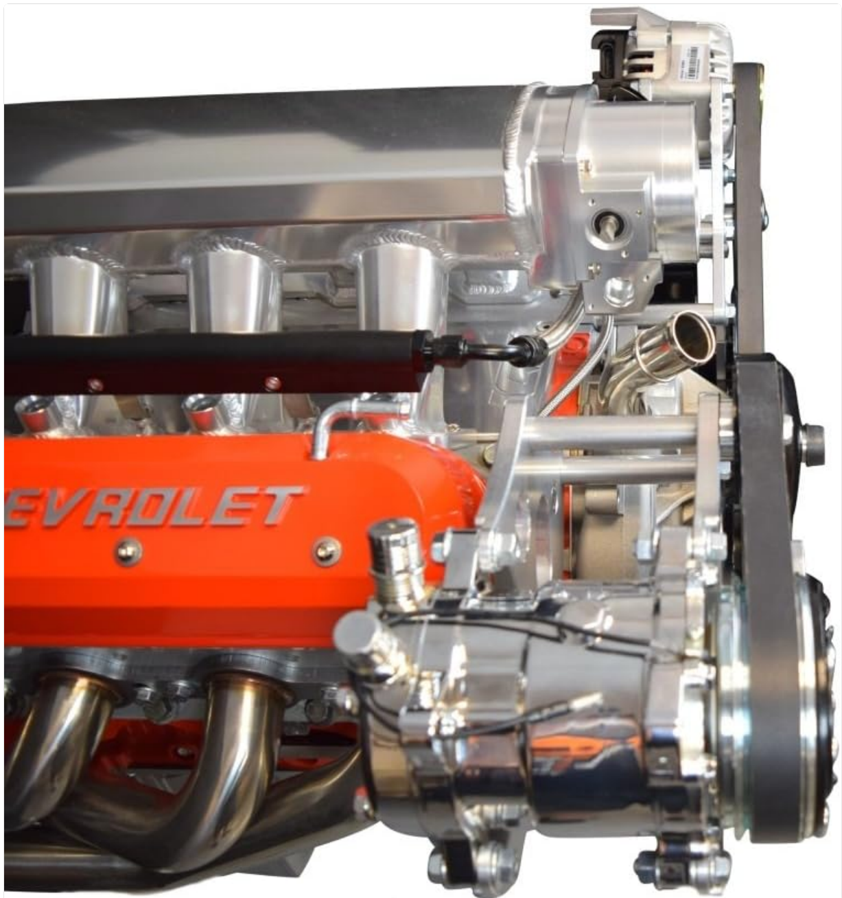
Image 4.2: Side view illustrating the compact design and how the bracket positions the A/C compressor relative to other engine accessories.
