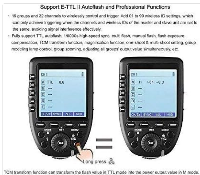
Figure 4: Display showing various flash modes and settings, including the TCM button for quick mode conversion.
