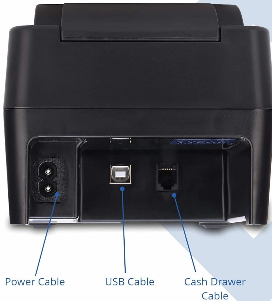
Image: Rear view of the Everycom EC-58 printer, highlighting the power cable port, USB cable port, and cash drawer cable port for easy identification during setup.
