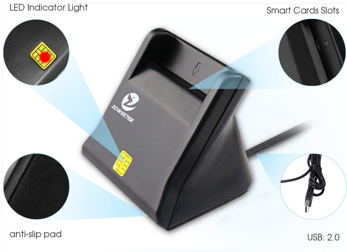
Figure 2: Key features of the ZOWEETEK CAC Smart Card Reader, including the LED indicator light, smart card slots, anti-slip pad, and USB 2.0 connectivity.
