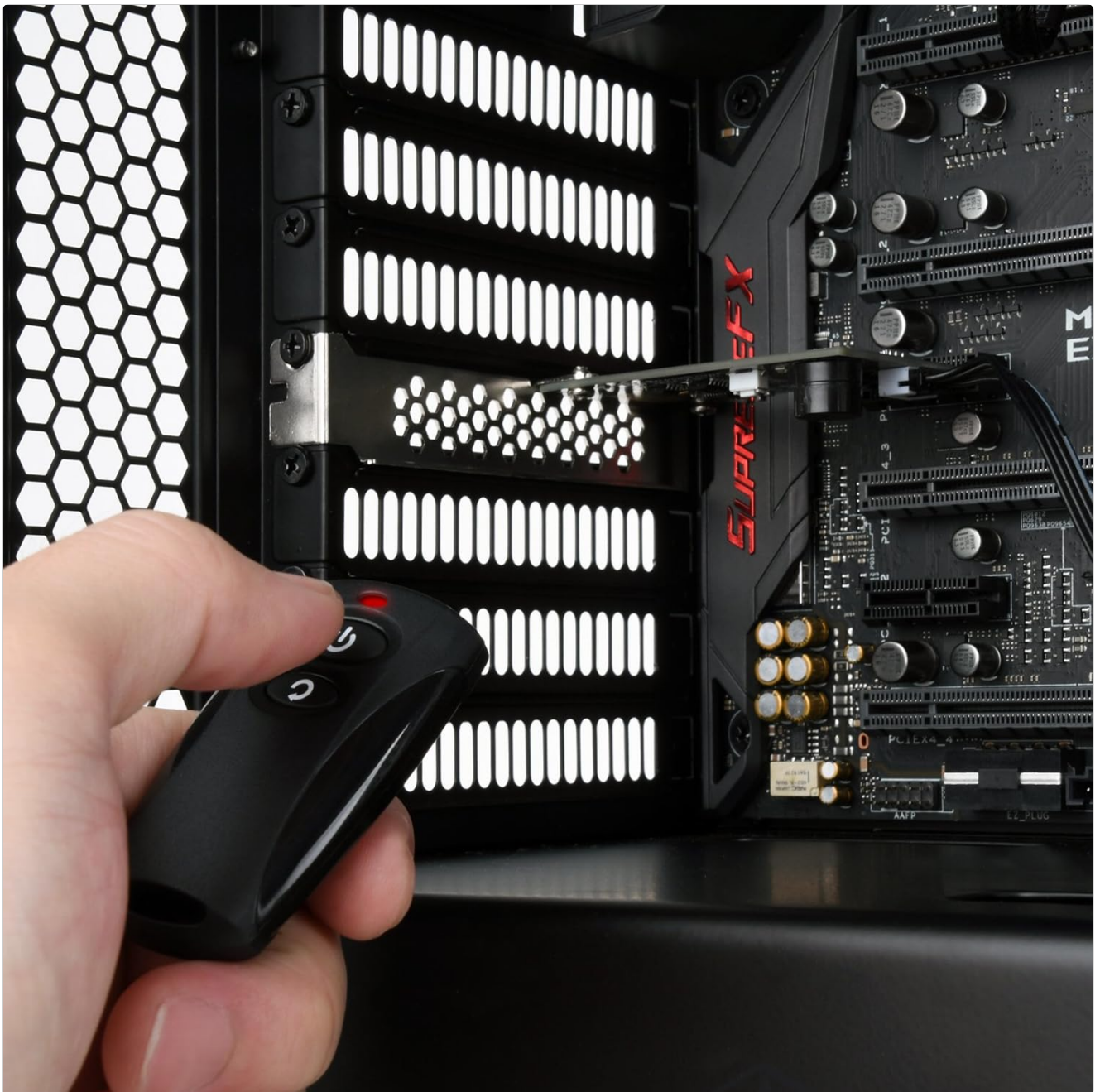
Image: A hand inserting the ES02-PCIE card into a PCI Express slot on a motherboard.
