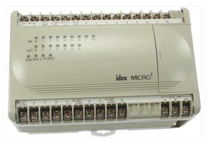
Figure 2.1: Front view of the FC2A-C16A1 Micro PLC. This image displays the various connection terminals, including power input (100-240 VAC), DC output (24V), DC input, digital inputs (IN 0-10), digital outputs (OUT 0-6), relay outputs (Ry OUT COM0, COM1, COM2), and data link terminals (A, B, SG). Indicator lights for Power (POW), Run (RUN), Error (E, R1, ERR2) are also visible.
