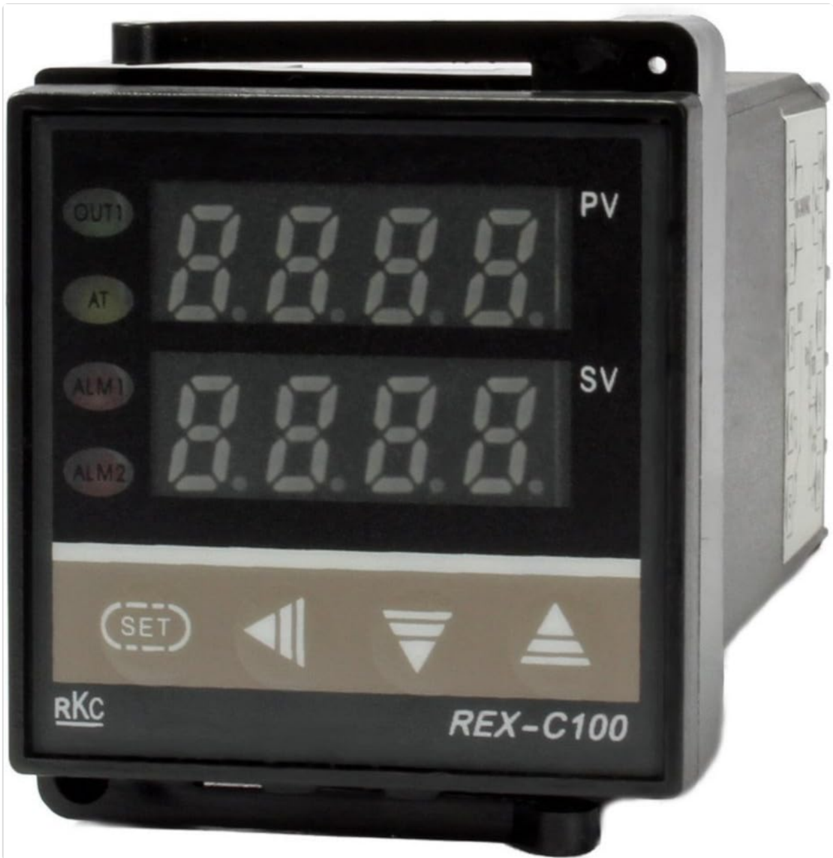
Figure 1: Front Panel of the RKC REX-C100 Temperature Controller. This image displays the controller's front face, featuring two digital displays for Process Value (PV) and Set Value (SV), indicator LEDs for OUT1, AT, ALM1, and ALM2, and control buttons for SET, Up, Down, and Left/Right navigation.
