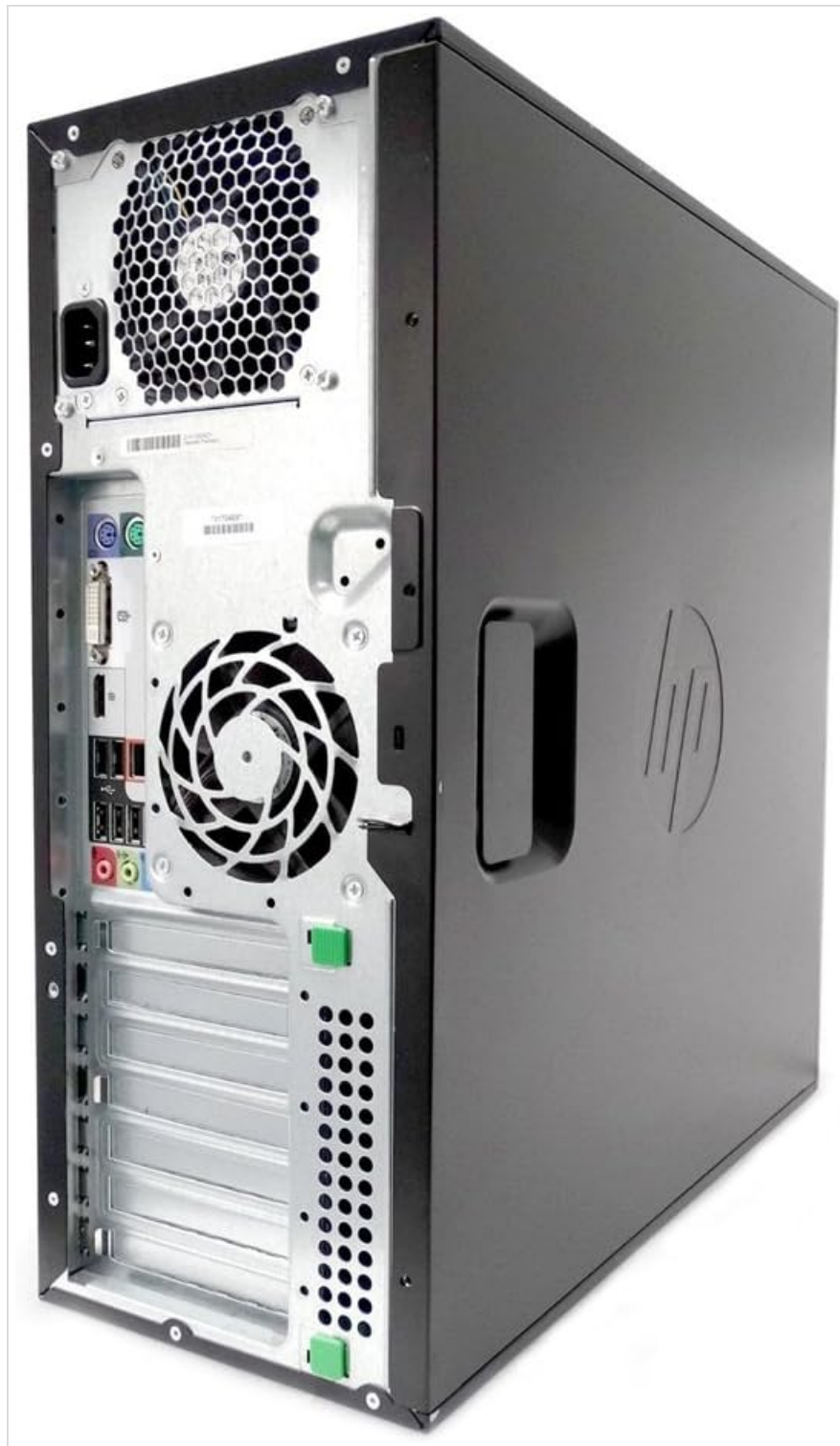
Image: Rear view of the HP Z210 Workstation Tower, displaying various ports including USB, audio, Ethernet, and video outputs.
